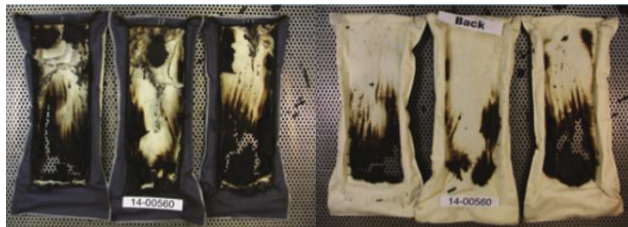
Front- exposed to arc flash
