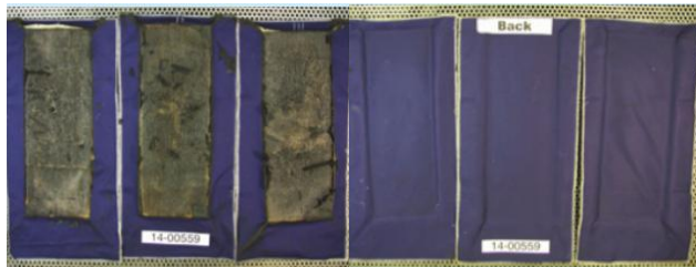
Front- exposed to arc flash
