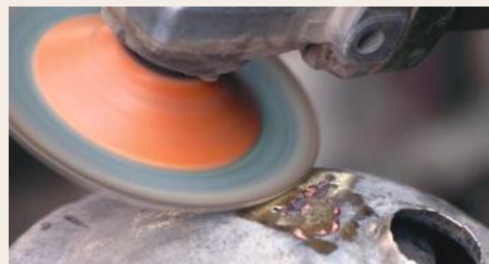
Craftsman polishing brass utensil- sourced from D-source
