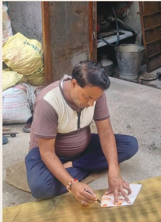
Craftsman marking shapes on the brass sheet - captured by Shruti Tiwari
