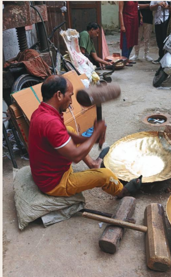
Craftsman hammering brass plate to give it a shape- captured by Gokulkrishnan
