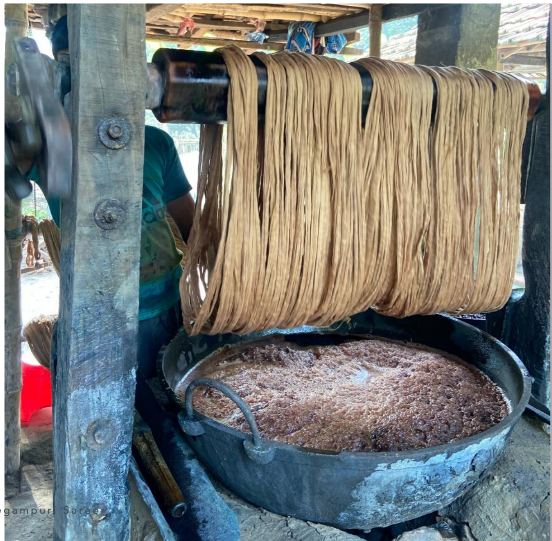
fig. 5.15 & 5.16 (above and below) cotton hanks being dyed
