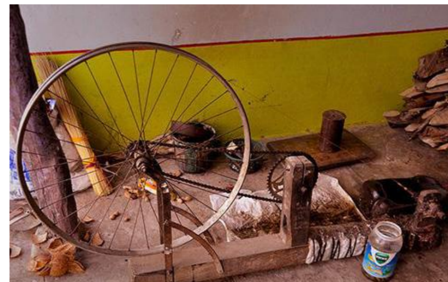
fig. 5.54 spinning wheel to make bobbins
