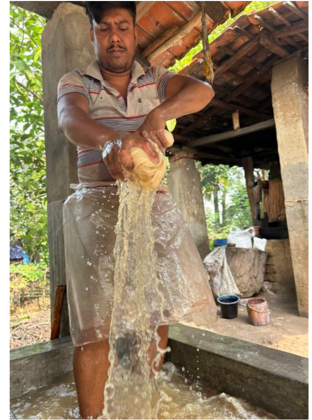
fig. 5.12 cotton hank bleaching process in H_2O_2
