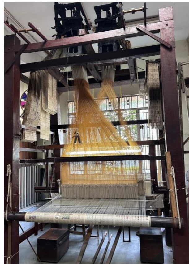
fig. 7.9 double jacquard box loom used in WSC Kolkata for Begampuri saree production
