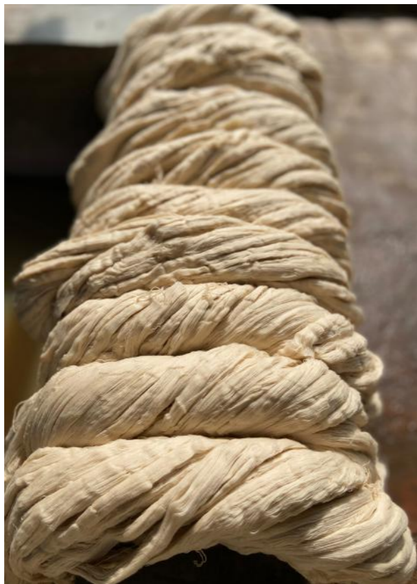
fig. 5.13 drying of bleached yarns
