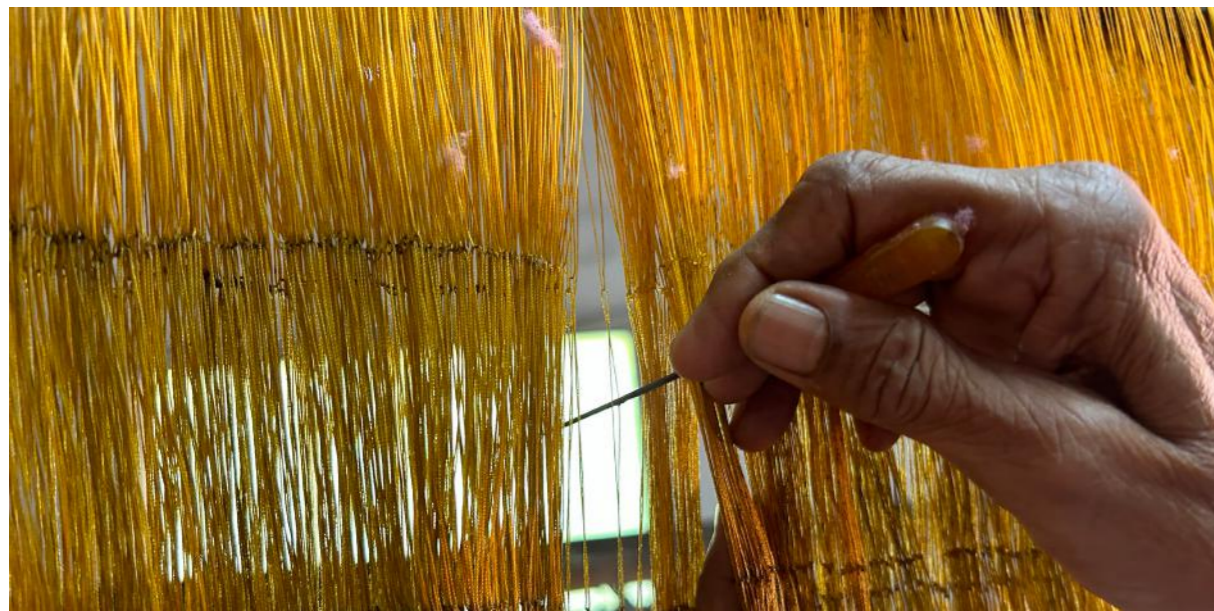
fig. 5.69 preparation of heald shafts
