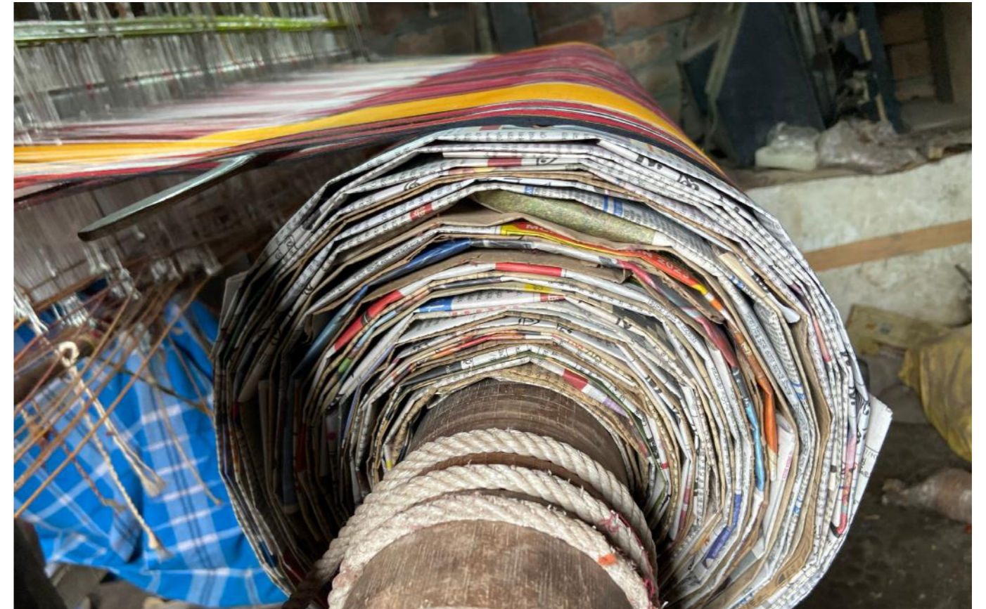
fig. 5.64-6.68 process of making a lease and warp beam through a drum roller
