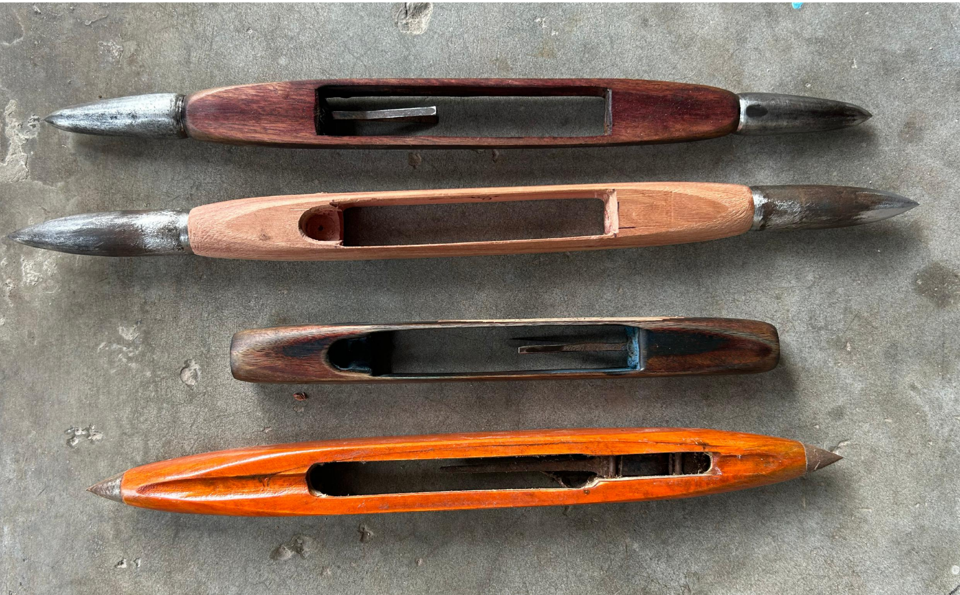
fig. 5.33 different kinds of shuttles used in both handloom and powerloom
