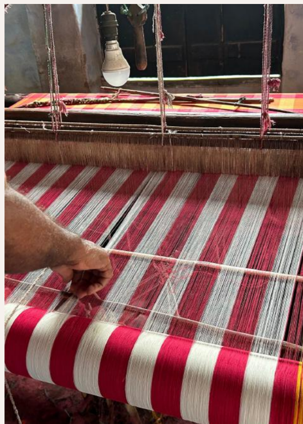
fig 5.84 fixing of broken yarns
