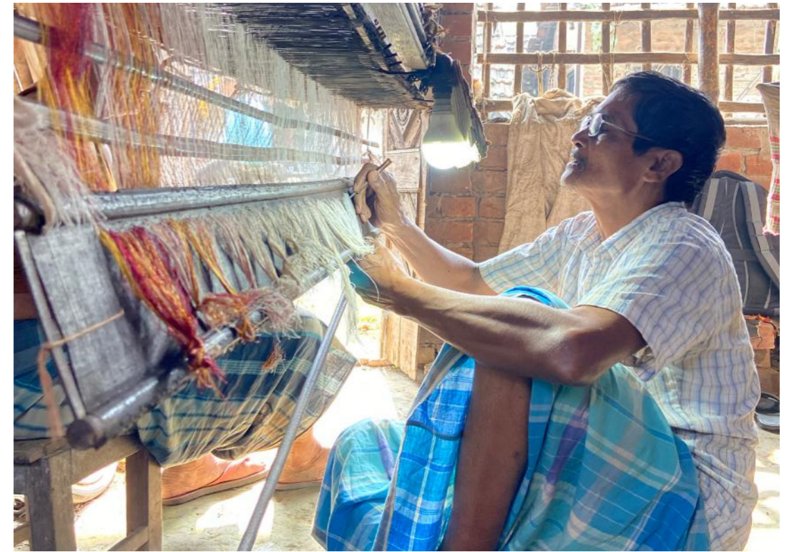
fig 5.74 denting of the yarns
