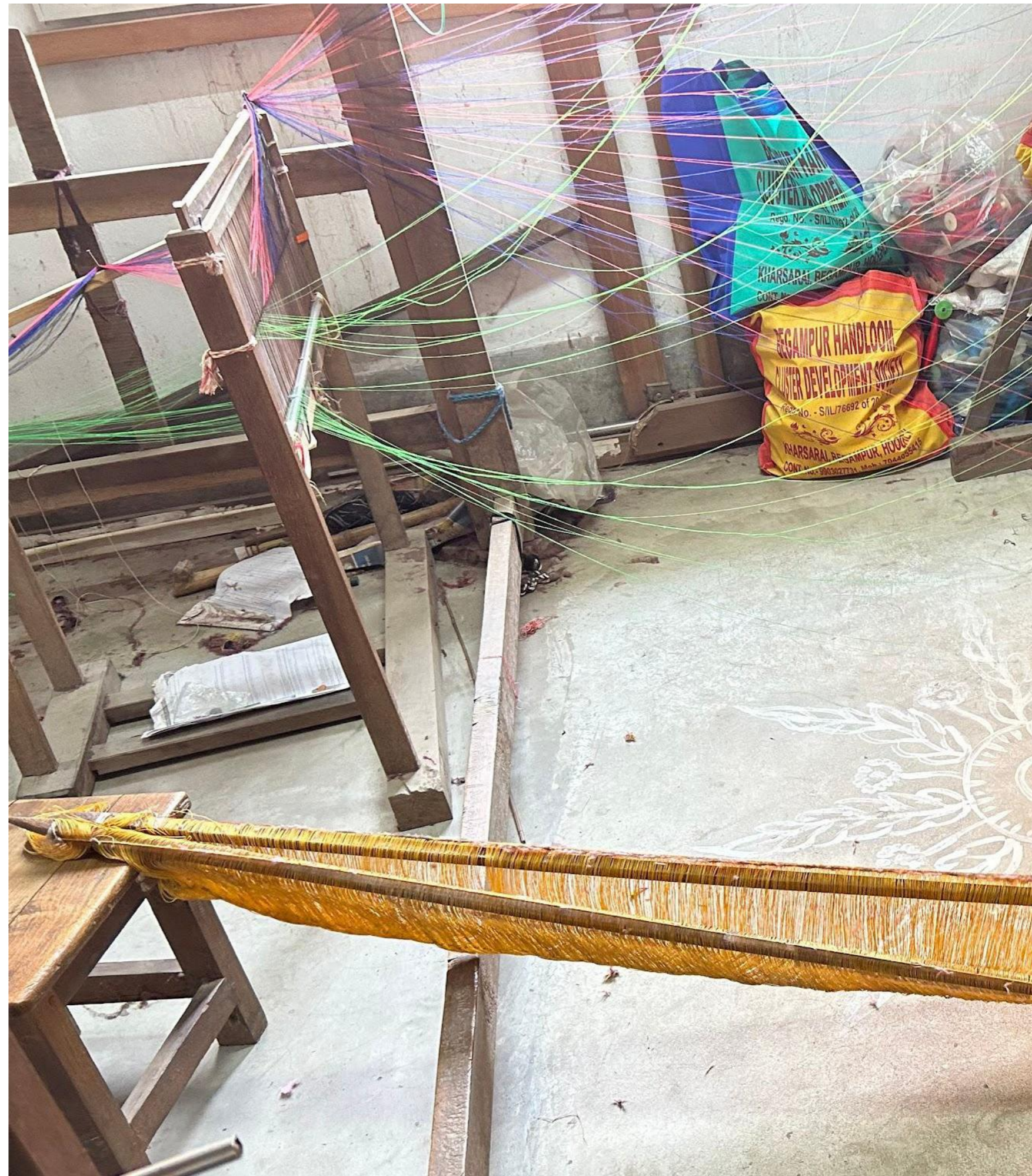
fig. 5.70 preparation of heald shafts
