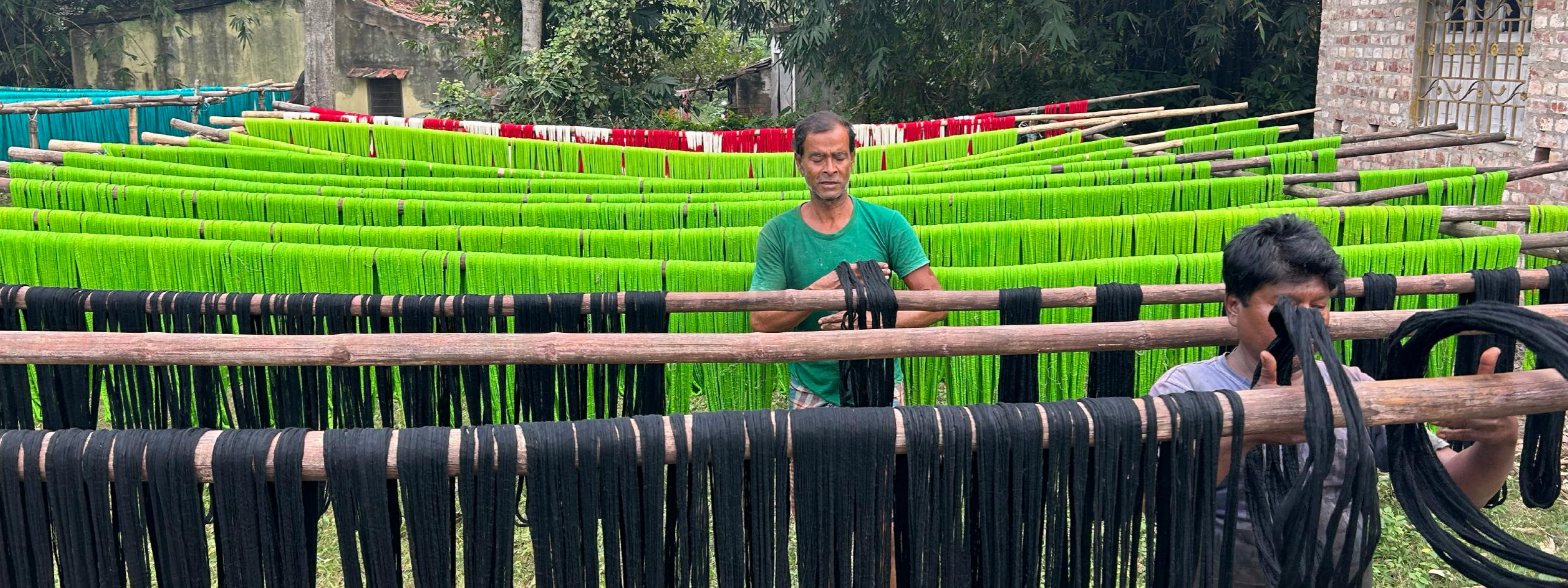
fig. 5.20 drying of dyed yarns
