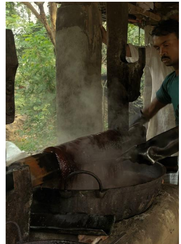
fig. 5.14 cotton hanks being dyed
