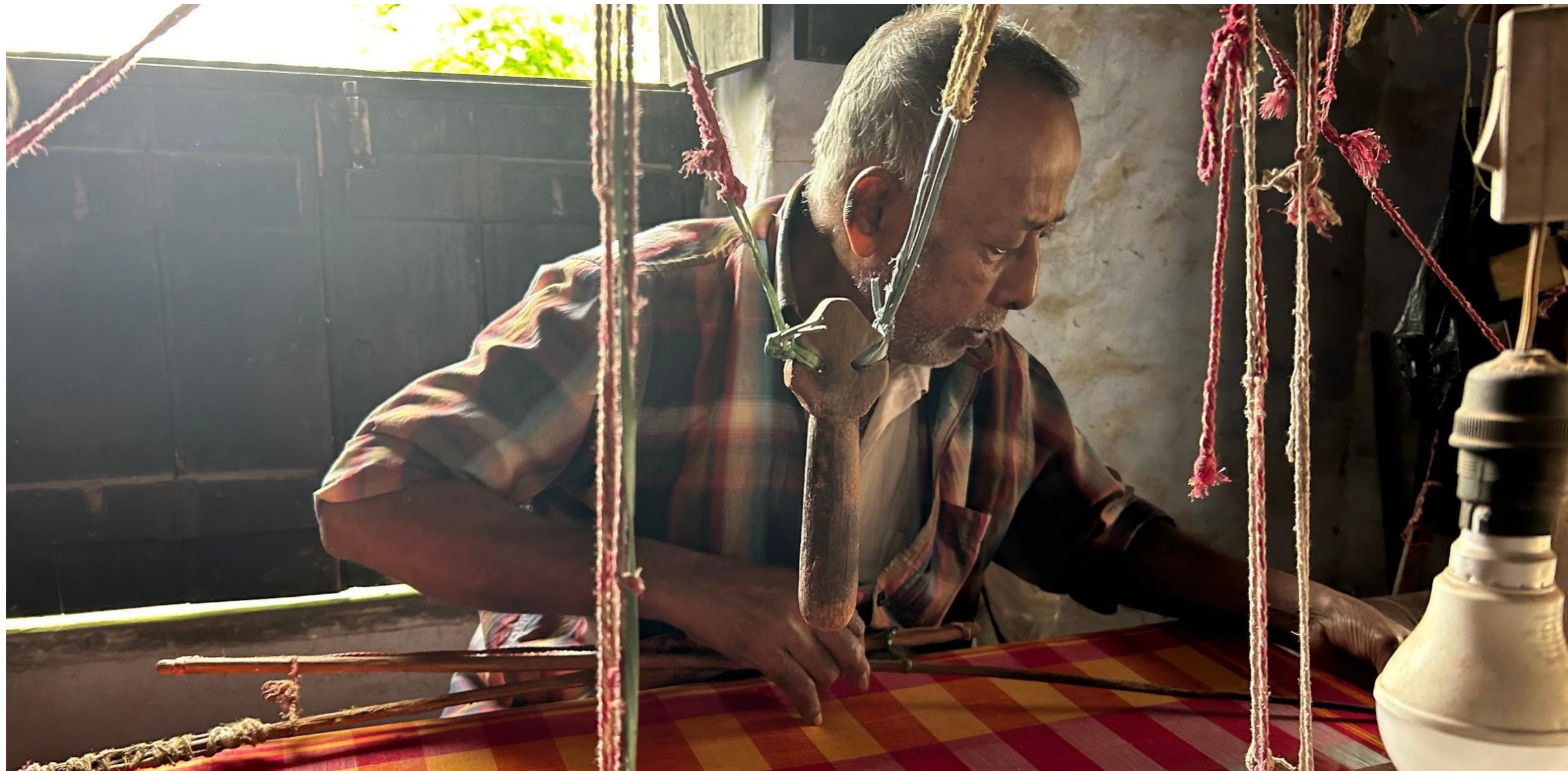
fig 5.75 (left) denting of the yarns fig 5.76 (above) weaving of the saree
