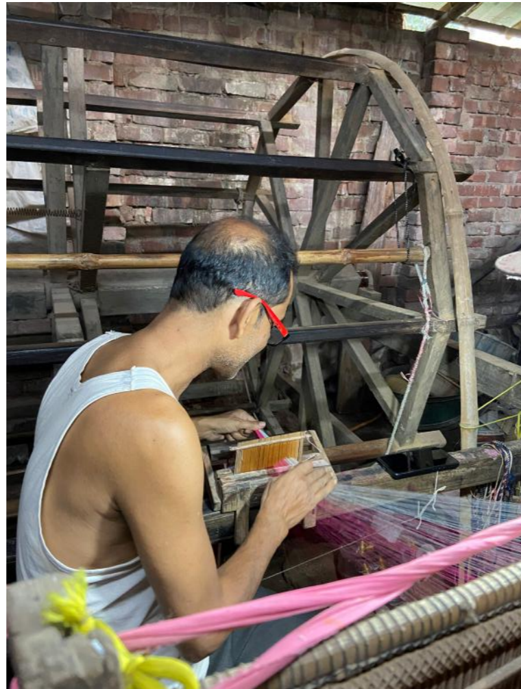
fig. 5.64-6.68 process of making a lease and warp beam through a drum roller
