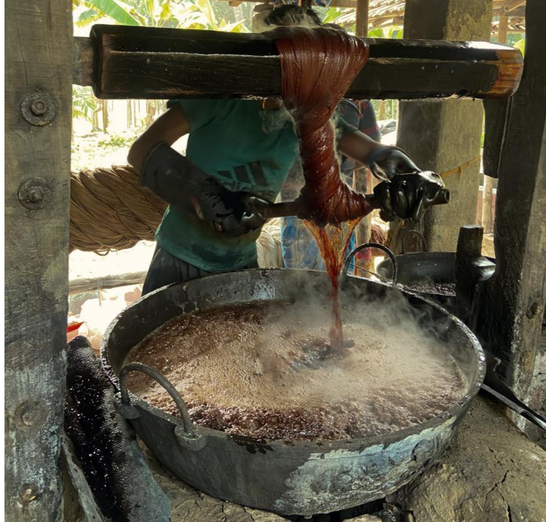
fig. 5.15 & 5.16 (above and below) cotton hanks being dyed
