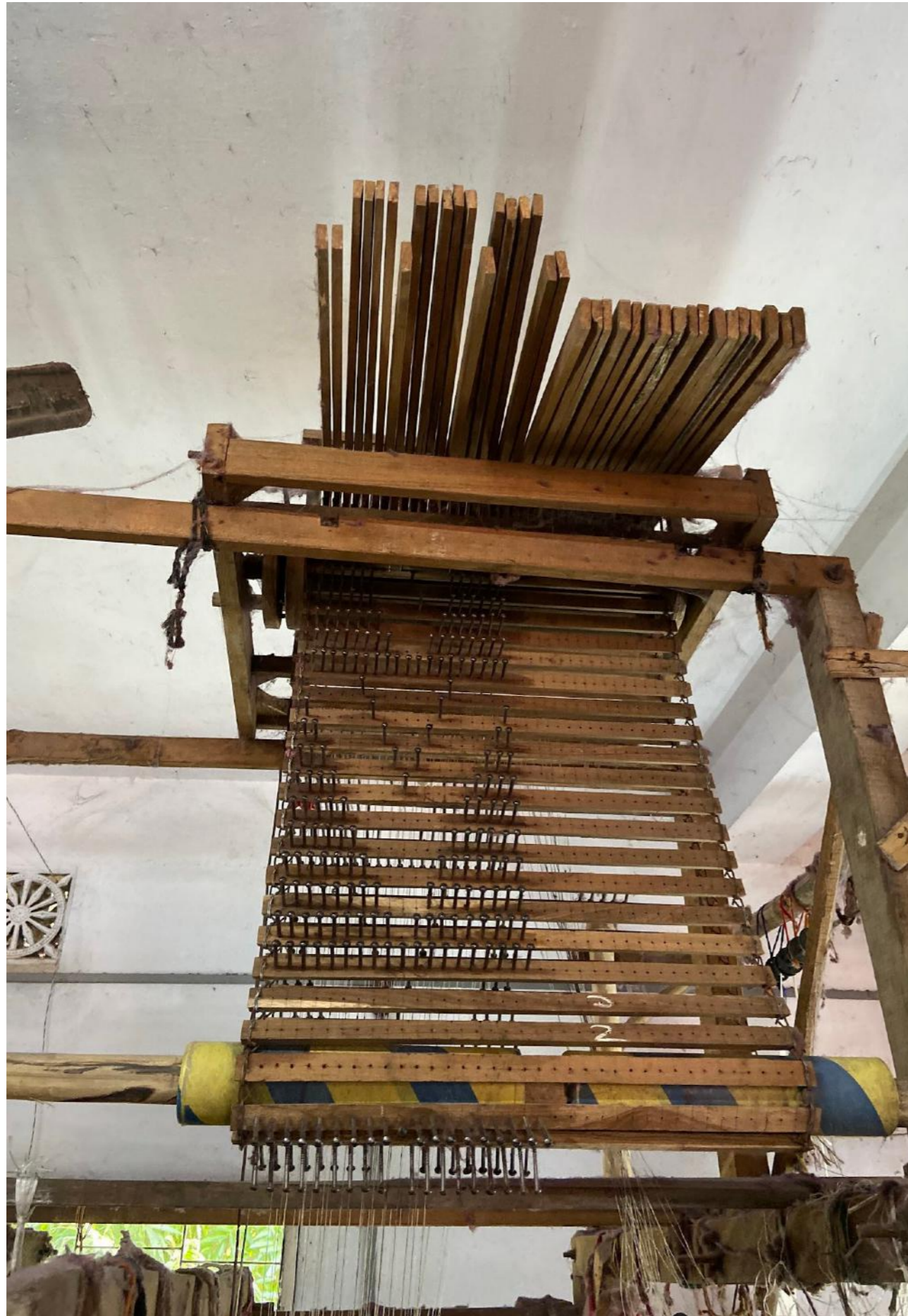
fig. 5.23 the dobby attachment on the loom
