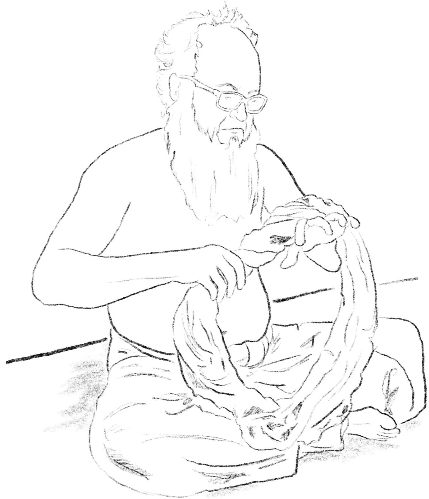
fig. 5.8 a man opening the hank for dyeing
