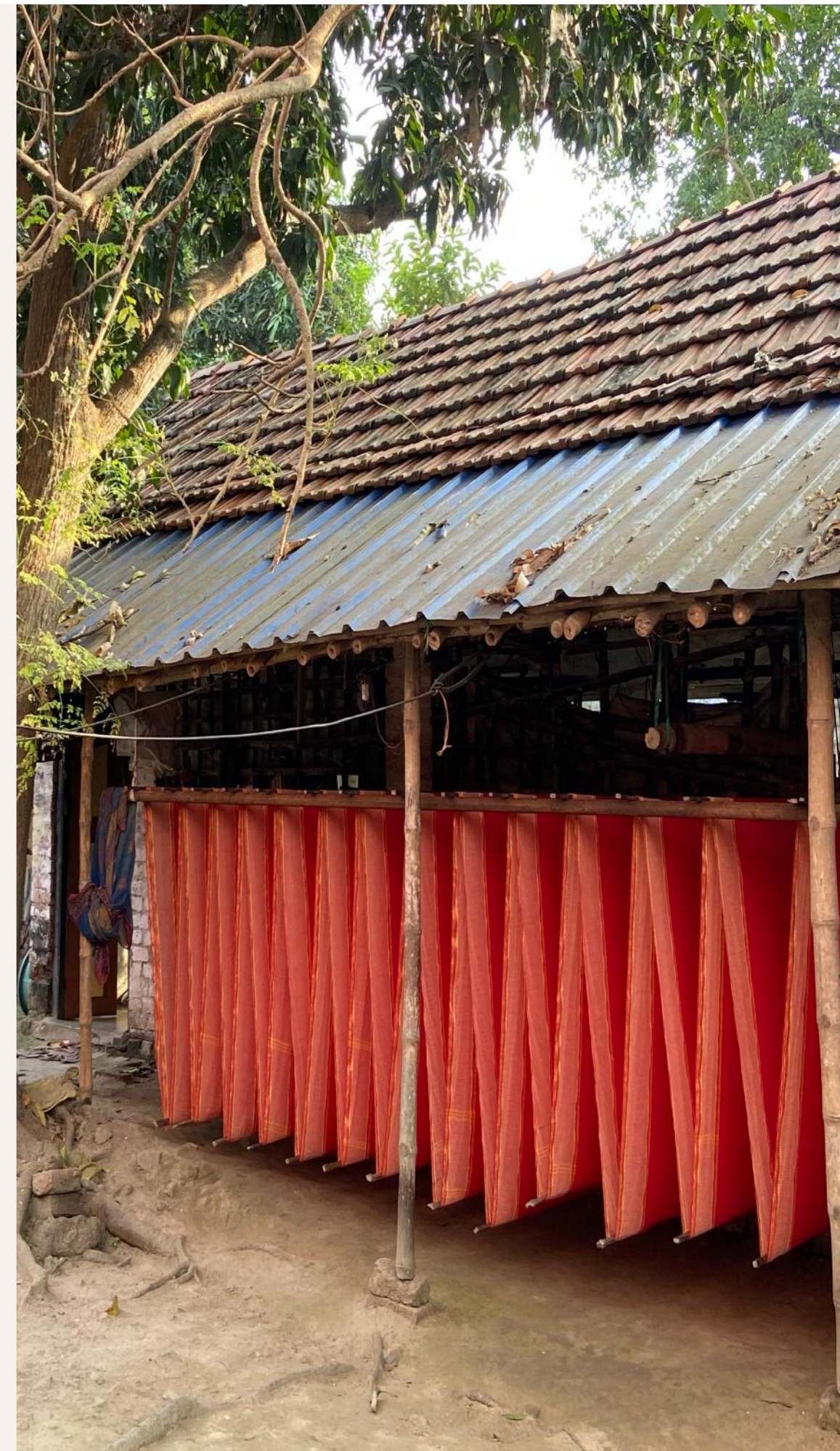
fig 5.86 drying of the starched sarees
