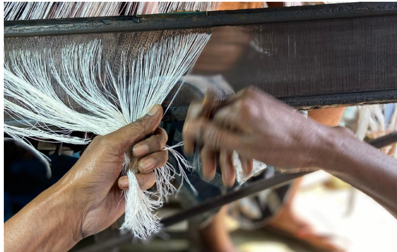
fig. 5.72 (left) setting of the warp beam for drafting fig 5.73 (above) denting of the yarns
