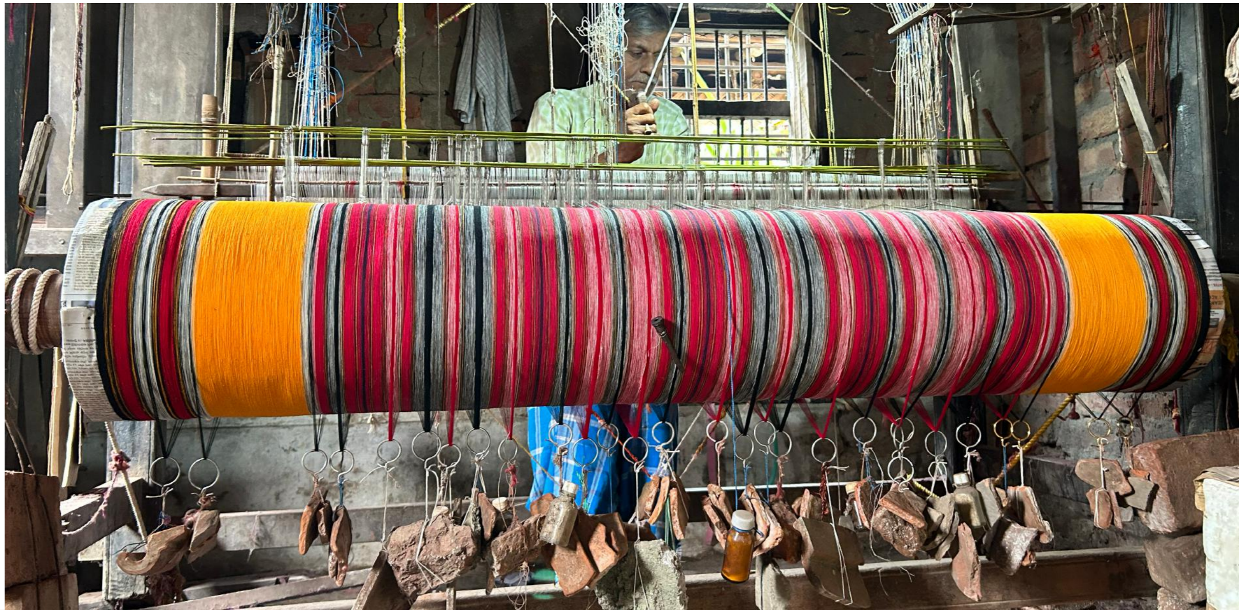
fig 5.81 different weights to manage extra warp
