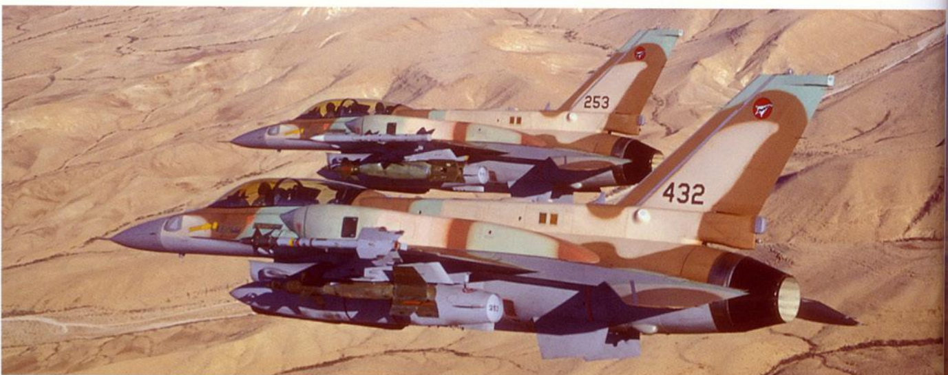
Aircraft numbers 253 (00-1004) and 432 (00-1017) of 'The Negev' squadron in formation over the southern desert of Israel. While F-16I number 253 payload includes 2,000 lbs. GBU-10 Paveway II Guided Bomb Units and AIM-120 AMRAAM air-to-air missiles, aircraft number 432 is armed with 500 lbs. GBU-12 Paveway I Guided Bomb Units and AIM-9L 'Sidewinder' air-to-air missiles. Photo: 'The Negev' squadron
