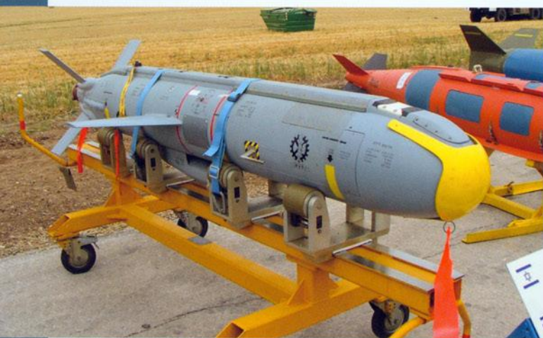
The Delilah 2 is actually a sophisticated EO cruise missile with a back-up GPS system. The missile, developed and produced by Israel Military Industries, incorporates a miniature warhead and is optimized to strike high value targets as it controlled by the WSO of the attacking aircraft. The RAFAEL produced data-link transceiver pod is positioned under the fuselage centerline pylon.
