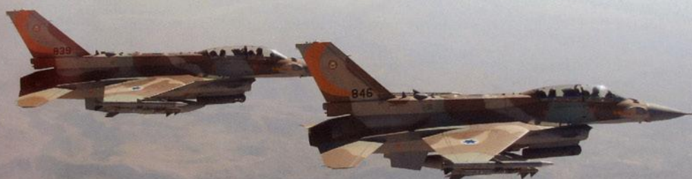
F-16I numbers 846 (99-9414) and 839 (99-9411), in formation flight over the Negev desert, configured for air-to-air missions with a payload of two 'Python 4' and two AIM-120 AMRAAM missiles and a single external fuel tank. Aircraft are without the conformal fuel tanks (CFT's). Photo: 'The Orange Tail' squadron
