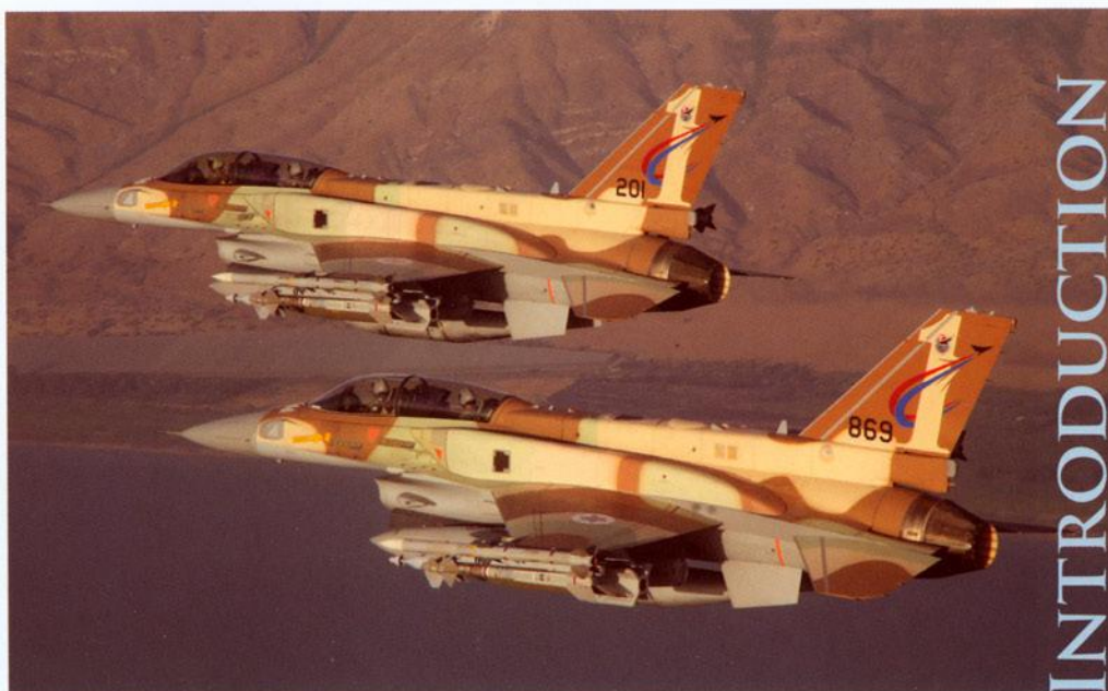
Above: A photo from an interesting angle of 'The Negev' squadron F-16I number 422 (00-1013), during flight. The aircraft is armed with two AIM-120 AMRAAM radar guided air-to-air missiles, two Python 4 infrared homing air-to-air missiles, two 2,000 lbs. GBU-10 Paveway II Guided Bomb Units, two 370 gallon external wing fuel tanks, one 300 gallon centerline fuel tank and a Litening II targeting pod and a Lockheed Martin LANTIRN navigation pod, positioned under the air intake.
