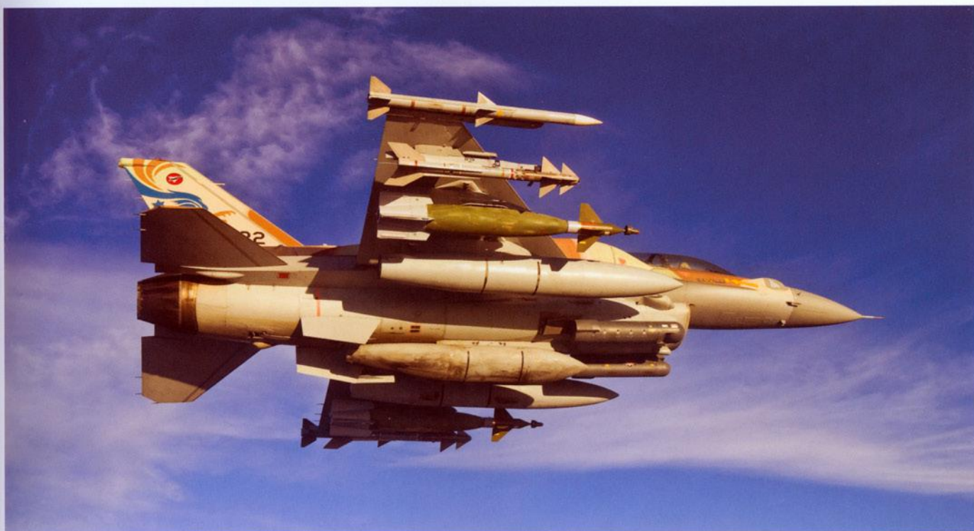
Above: A photo from an interesting angle of 'The Negev' squadron F-16I number 422 (00-1013), during flight. The aircraft is armed with two AIM-120 AMRAAM radar guided air-to-air missiles, two Python 4 infrared homing air-to-air missiles, two 2,000 lbs. GBU-10 Paveway II Guided Bomb Units, two 370 gallon external wing fuel tanks, one 300 gallon centerline fuel tank and a Litening II targeting pod and a Lockheed Martin LANTIRN navigation pod, positioned under the air intake.
