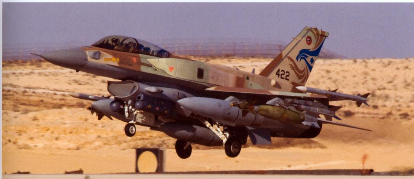
Below: F-16I number 422 (00-1013), taking off in a similar configuration of number 407 seen on the right. Payload also consists of a LANTIRN navigation and a Litening II targeting pod.
