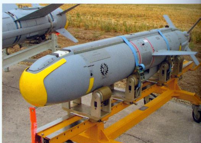
The Delilah 2 is actually a sophisticated EO cruise missile with a back-up GPS system. The missile, developed and produced by Israel Military Industries, incorporates a miniature warhead and is optimized to strike high value targets as it controlled by the WSO of the attacking aircraft. The RAFAEL produced data-link transceiver pod is positioned under the fuselage centerline pylon.
