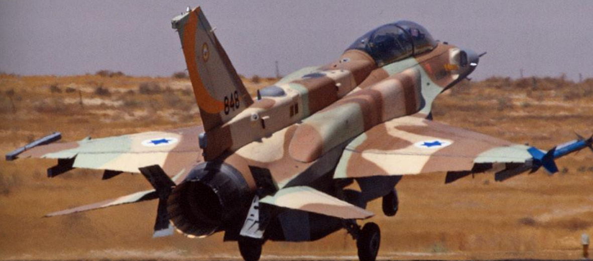
Aircraft number 848 (99-9415) landing at Hatzerim AFB, returning from an air-to-air training sortie with an AIM-9L Sidewinder training missile and a 300 gallon centerline external fuel tank. Photo Ofer Zidon
