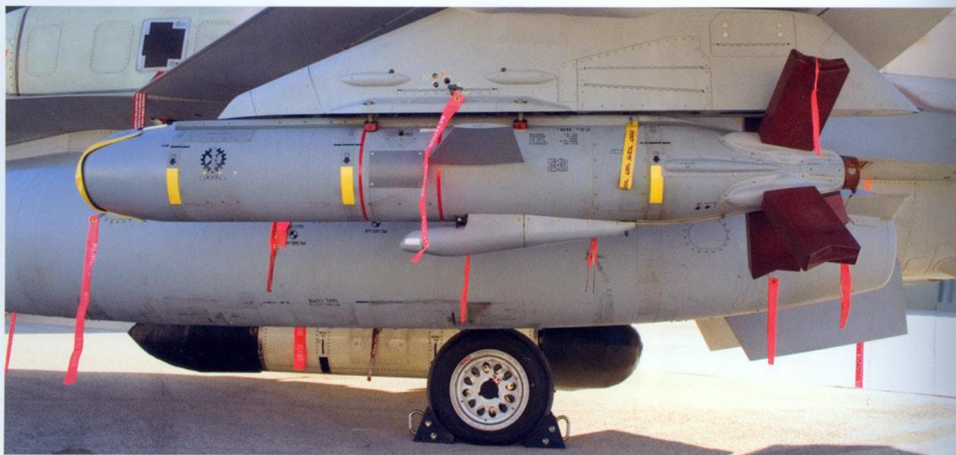
The Delilah 2 is actually a sophisticated EO cruise missile with a back-up GPS system. The missile, developed and produced by Israel Military Industries, incorporates a miniature warhead and is optimized to strike high value targets as it controlled by the WSO of the attacking aircraft. The RAFAEL produced data-link transceiver pod is positioned under the fuselage centerline pylon.
