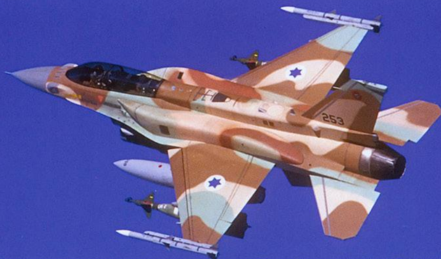
F-16I number 253 (00-1004), during a turn, revealing the upper camouflage scheme of the aircraft including that of the conformal fuel tanks (CFT's). Clearly visible is the different shade of brown on the CFT's, that were painted in Israel, compared to the brown that was applied to the aircraft.
