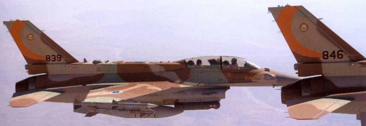
Aircraft numbers 846 (99-9414) and 839 (99-9411), in formation flight over the Negev desert, configured for air-to-air missions with two 'Python 4' and two AIM-120 AMRAAM missiles and a single external fuel tank. The aircraft are lacking conformal fuel tanks (CFT's). Photo: 'The Orange Tail' squadron
