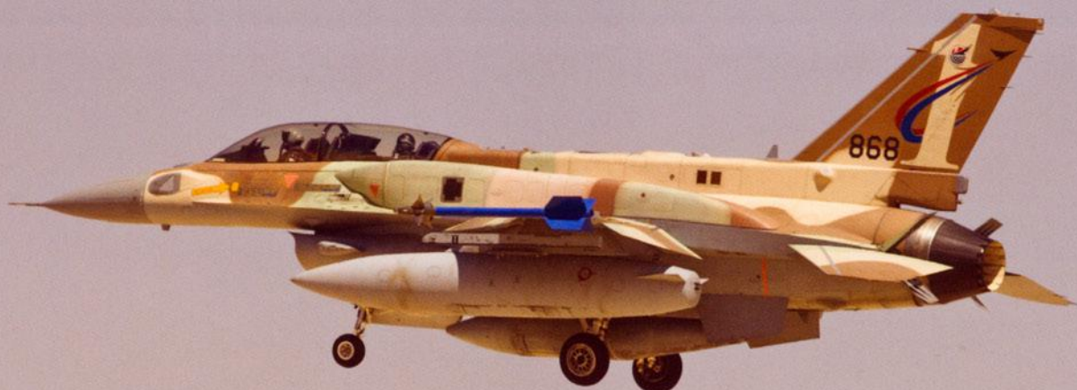
Aircraft number 868 (99-9428) on landing approach after training sortie. Of note are the under-wing Israel Military Industries 600 gallon external fuel tanks and the open split trailing edge airbrakes.
