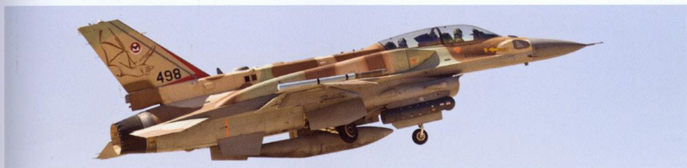
Above: Aircraft number 498 (99-9412) taking-off taking-of to an air-to-air training sortie. Of note is the RAFAEL Litening II pod. This F-16I was due to receive the IAF number 843, but its number was already changed at the Lockheed Martin plant in the U.S.A.
