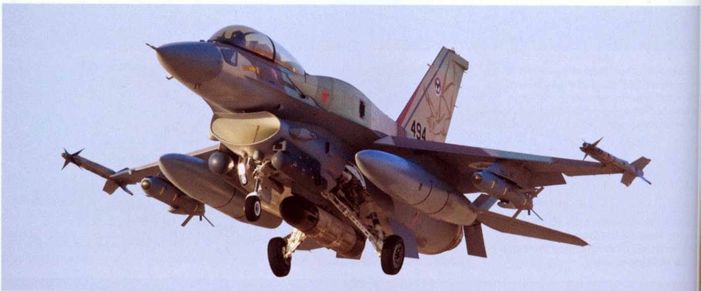
Aircraft number 494 (00-1048) taking-off with a payload of two AIM-9L 'Sidewinder' air-to-air missiles, two 'Delilah' missiles, a pair of 370 gallon external fuel tanks and a 'Delilah' data link pod on the fuselage centerline pylon. Also carried are the guidance and targeting pods under the air-intake. Below is the same aircraft on landing approach. Above photo: Tal Shoham
