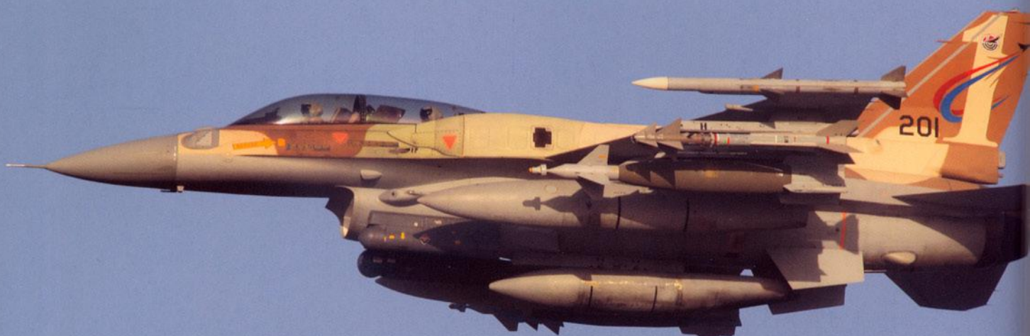
The 'Flagship' aircraft of 'The One' squadron, F-16I number 201 (99-9426) in flight, with a heavy payload that consists of three external fuel tanks, the AN/AAQ-13 LANTIRN navigation pod, the RAFAEL Litening targeting pod, two 'Python 4' IR and two AIM-120 AMRAAM radar guided missiles. Two 2,000 lbs GBU-10 Paveway II Guided Bomb Units. Noteworthy are the grey warhead and control sections of the bombs typical to Lockheed Martin kits. The Raytheon kits are painted olive drab. Photo: 'The One' squadron
