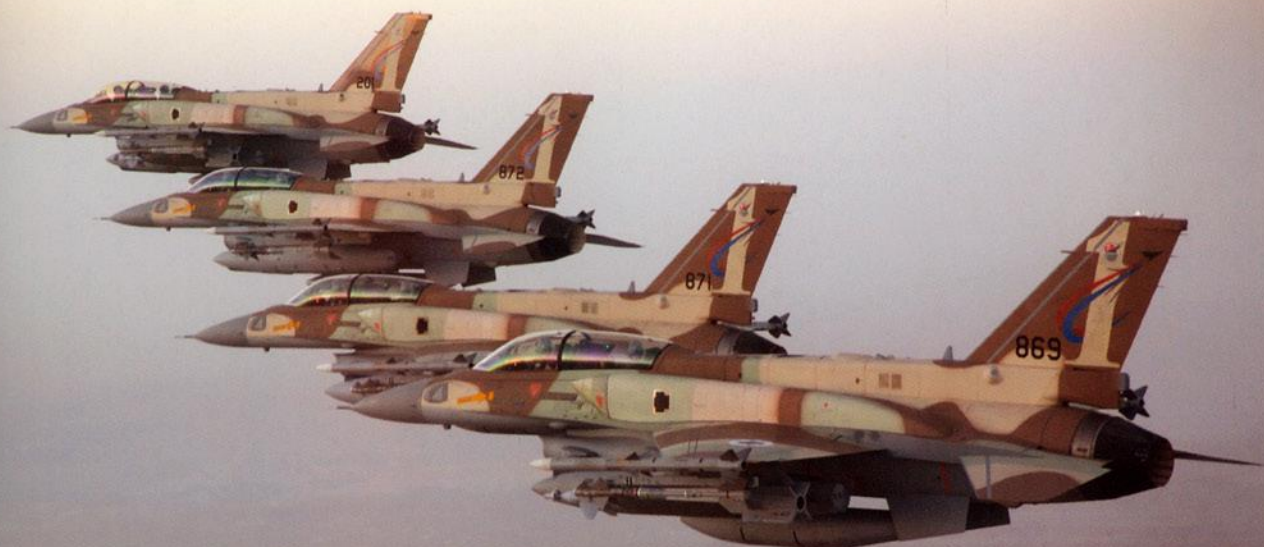
Aircraft numbers 869 (99-9429), 871 (99-9430), 872 (99-9431) and 201 (99-9426) in formation, all with a payload of 'Python 4' and AIM-120 AMRAAM air-to-air missiles, while only numbers 869 and 201 are also armed with laser guided bombs (LGB's).
