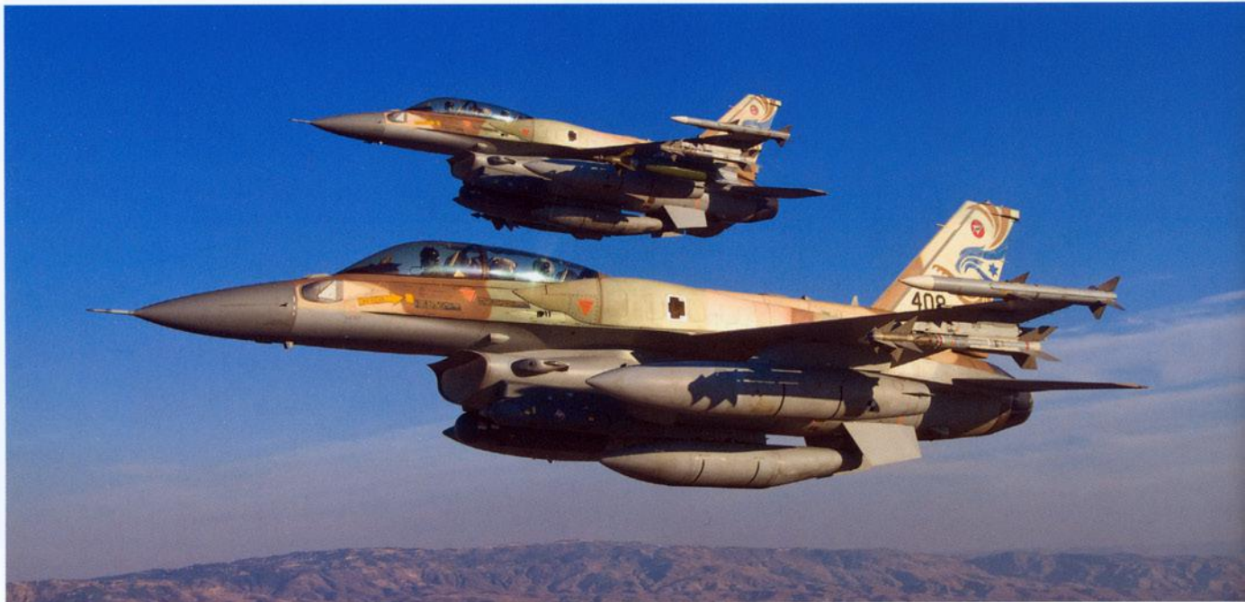
Above: 'The Negev' squadron aircraft numbers 407 (00-1005) and 408 (00-1006) with a payload of AIM-120 AMRAAM and Python 4 air-to-air missiles and three external fuel tanks. Aircraft number 407 is armed with two 2,000 lbs. GBU-10 Paveway II Guided Bomb Units.
