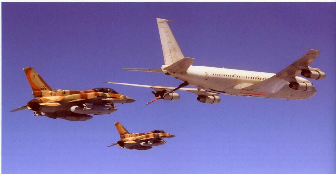
Above: Aerial refueling is common practice for IAF pilots. Illustrated in this photo are 'The Orange Tail' squadron aircraft numbers 803 (99-9401) and 836 (99-9410) approaching an IAF 'Re'em' (Hebrew for an Oryx) Boeing 707 tanker. The F-16s are armed with Laser Guided Bombs, two 600 gallon under wing and a 300 gallon centerline external fuel tanks.
