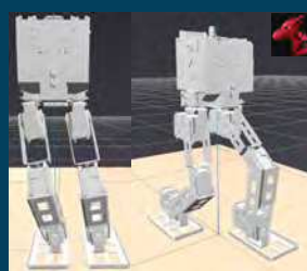
Inverse pose kinematics validation in Drake
