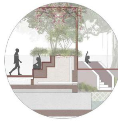
Retaining Wall of the Canal used for Seating and Planting
