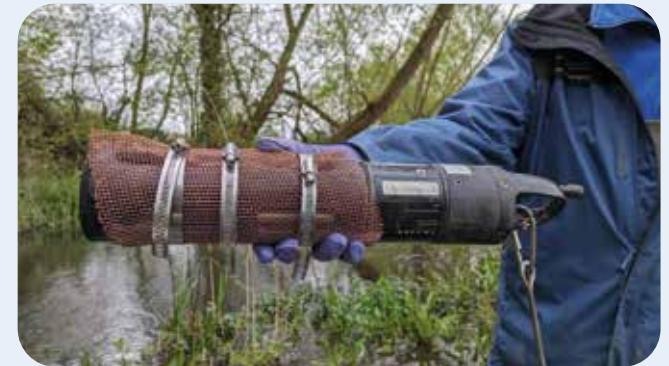
Protective copper mesh around a sonde to prevent fouling by sediment and algae
