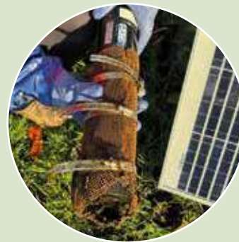
Sondes are powered by solar panels
