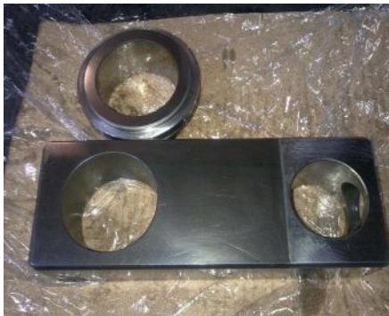
API Slab gate
