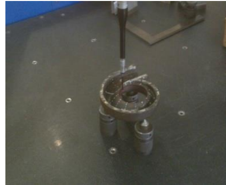
Fig 4. Measurement of interior profile of casing on CMM
