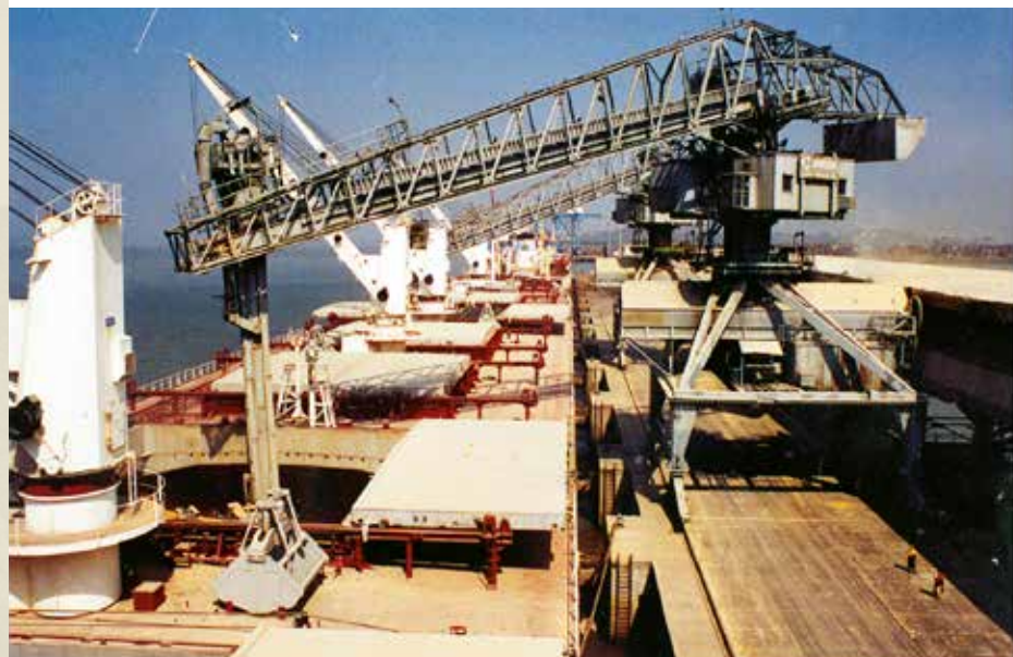
Continuous unloaders installed at the bulk terminal for bulk cargo handling. The bulk terminal was later demolished to make way for a new container terminal
