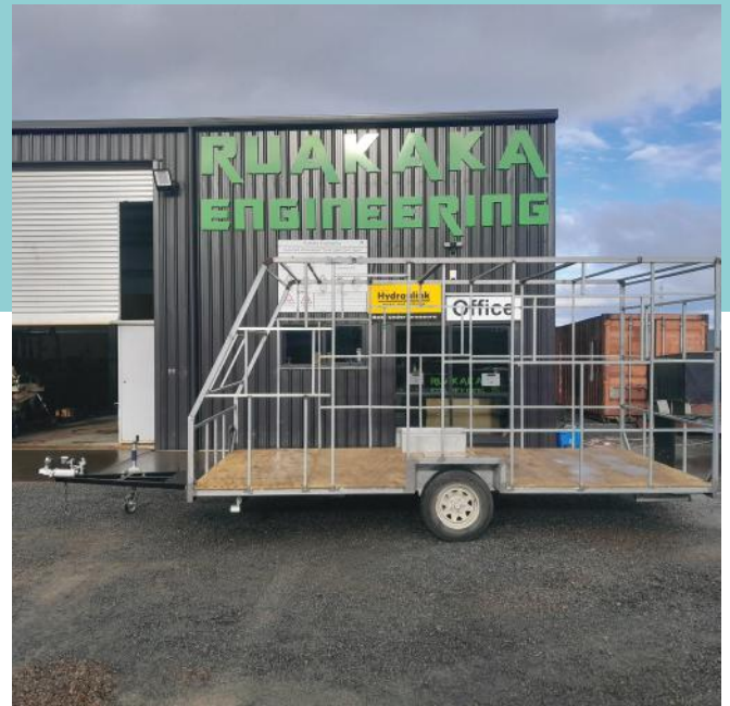
Braedon Kenny made a Caravan trailer. He did all the welding at Ruakaka Engineering and the trailer has passed a WOF.
