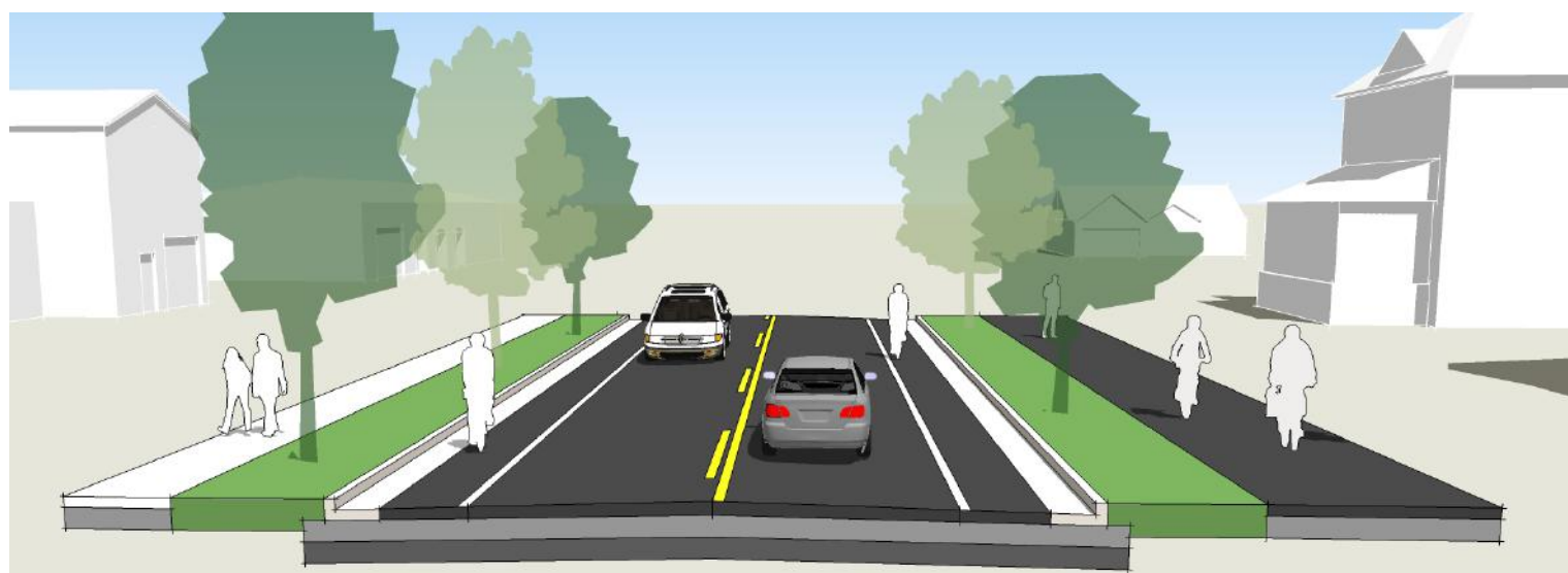
Figure 3.23: Example Local Road Typical Section with Shared Use Path and On-Street Bicycle Lanes (Mead & Hunt, Inc.) from the Town of Ledgeview Bicycle & Pedestrian Master Plan 2019
