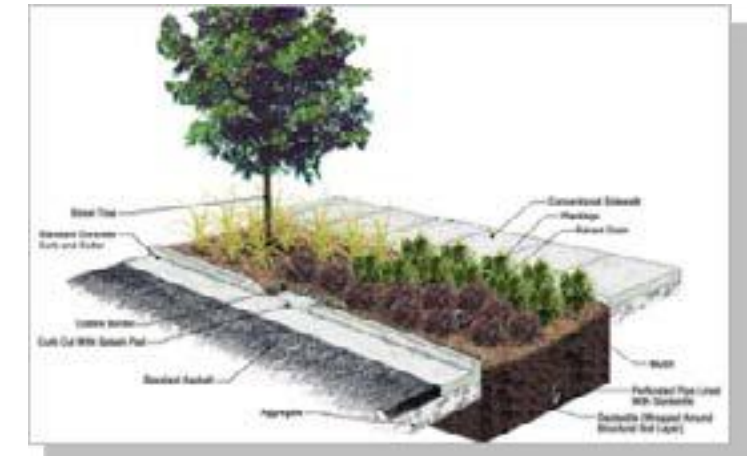
Figure 6.3: Bioswale Diagram. Source: Source - City of Milwaukee Green Streets Stormwater Management Plan
