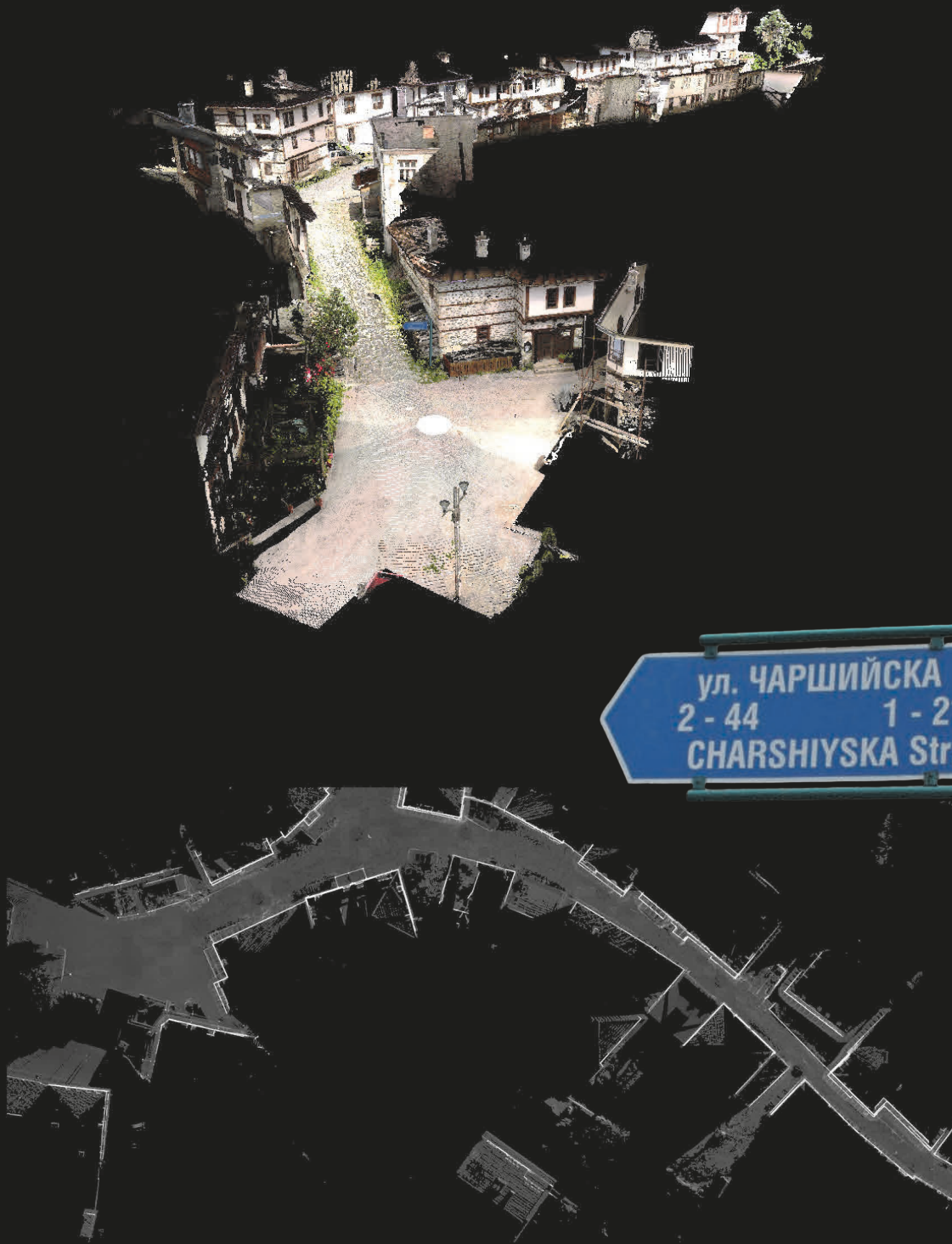
Figure 30-31: (Above) Final 3D model of Charshiyska street (Right) 3D scanning as a survey of the current state of cultural monuments and those at threat along it (Authors own, 2025)
