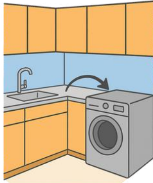
Image – Appliances in corner block access
