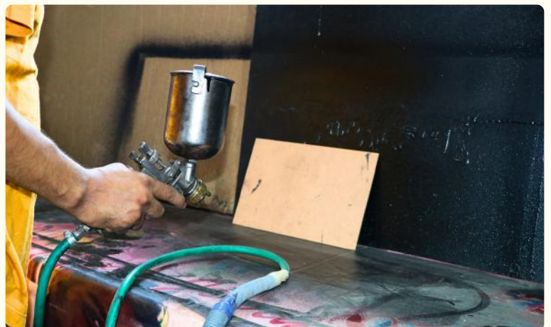
Fig 3.2.3 : Process of base coating the MDF board
