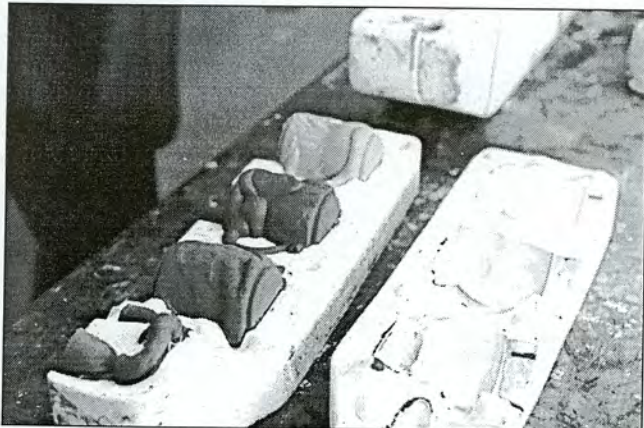
Pouring of animal mugs in a mould
