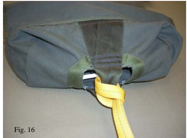
Turn the bag right side out. Be certain that all of the apex lines are inside the bag. (fig.#16)
