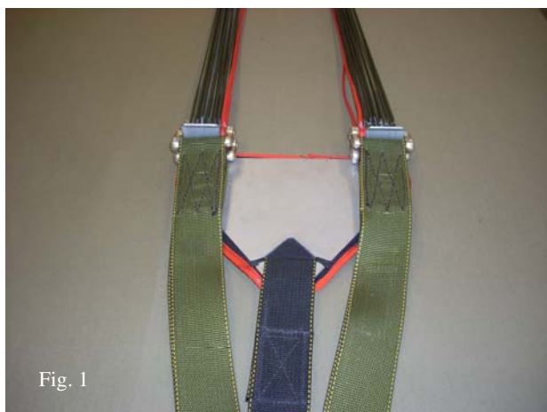
Fig. 1 Lay the canopy on the table or floor with the risers flat, not twisted and links on the tension plate. (fig. # 1)
