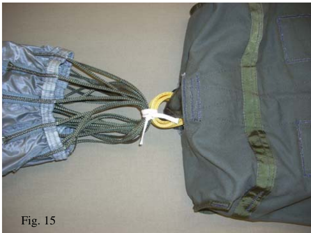
Trim the #80 Cotton Break-tape leaving an inch to two inches (1-2") of tail. (fig.#15)
