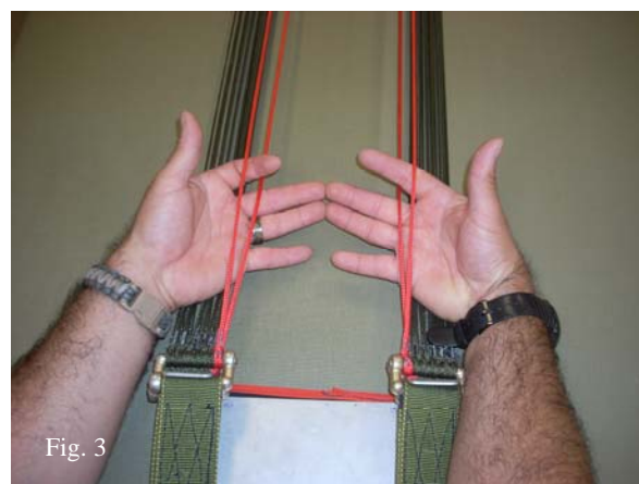
Fig. 3 Check suspension lines for proper layout using four-line check method. (fig. # 3)
