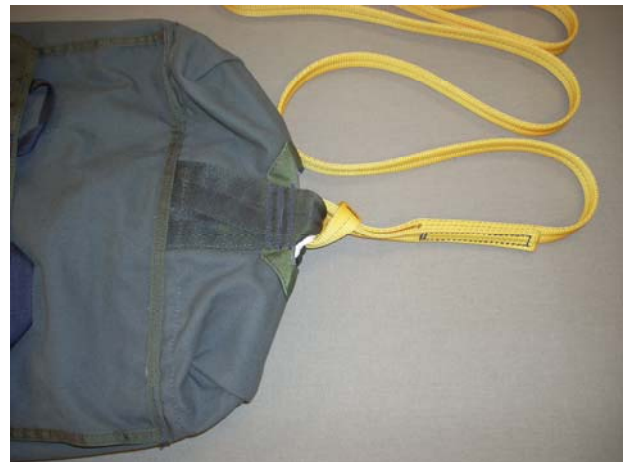
Turn the bag right side out. Be certain that all of the apex lines are inside the bag. (fig.#16)
