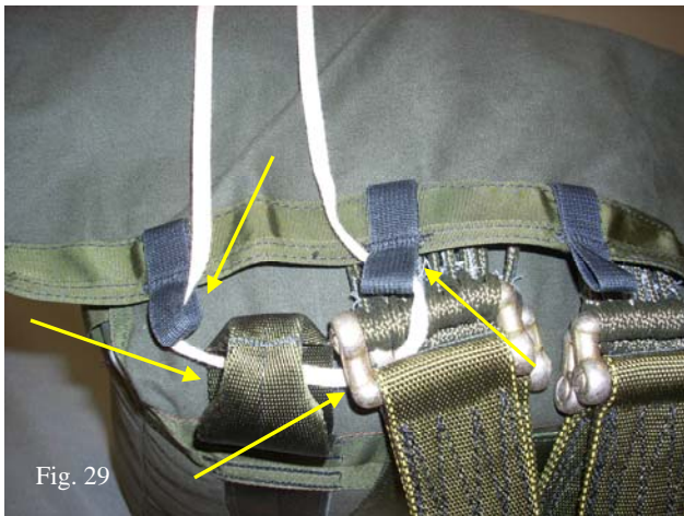
Pass a length of 80# break-tape through the 5/8" T-4 loop, the T-8 loop, both connector links then the 5/8" T-4. (fig. #29)
