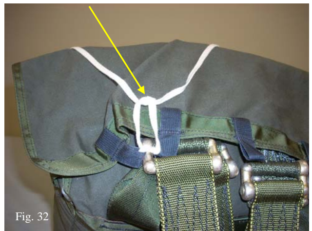
Tie an Over-hand knot. (fig. #32)
