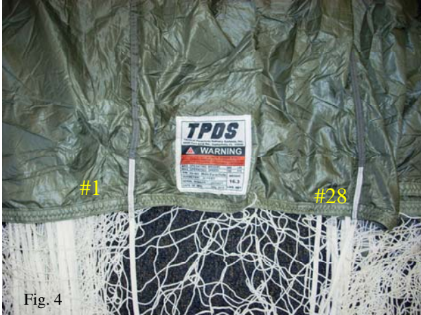
Pictured above is the top of the HURP Parachute with data placard. (fig. #4)
