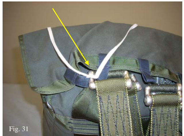
Tighten the knot formed. (fig. #31)
