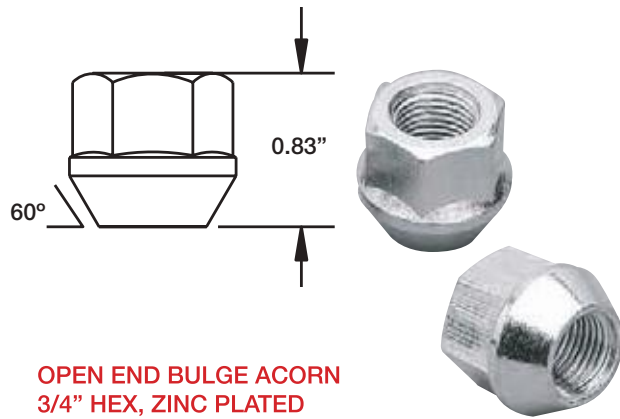
HEAT TREATED OPEN END BULGE ACORN 3/4" HEX, ZINC PLATED
