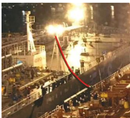
Correct lift for drainage
