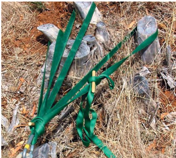
The picture above shows a 3x1 on three freshly cut olive trees where the rigger used small wood dowels as crush elements to allow an airspace in the fixing knot for ease of untying.
