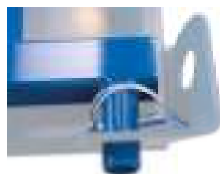
Securing the tipping unit to the steel-frame dolly with linchpins
