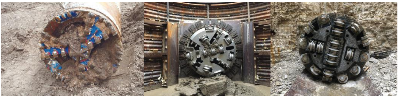
Examples of cutterhead types: (Left to Right) Soft ground, Mixed Ground, Rock
