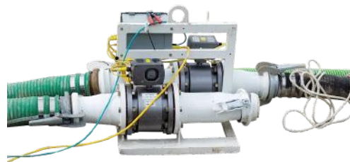
Figure 4.10: Magnetic type slurry flow meters. Non-density type meters.
