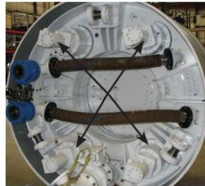
Main drive hydraulic motors and gear boxes (4)
