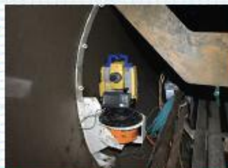
Pipe Station with adjustable pipe ring and hinged blocker plate to prevent false prism readings
