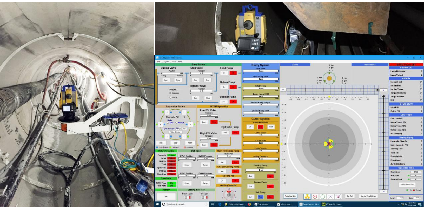
Figure 4.12: General Arrangement of Akkerman AZ-100 Total Guidance System Set-up.
