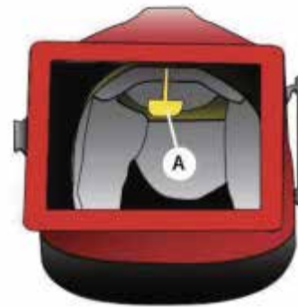
Air flow < 165 dm 3 /min - indicator protruding
