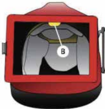
Air flow > 165 dm 3 /min - indicator tucked in
