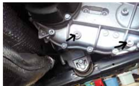
The fill (left) and drain (right) plugs on transfer case:
