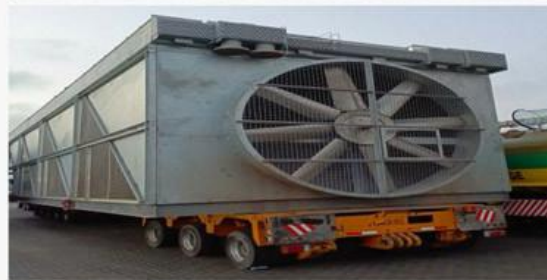
Exhaust : 50 tons, Dimensions 18.28 * 3.96 * 4.27 M
