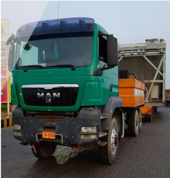
Exhaust : 50 tons, Dimensions 18.28 * 3.96 * 4.27 M
