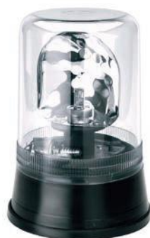
AEB "595" BEACON LIGHT 24V Clear lens, height 220mm, Ø 160mm 3-bolt mount, H1-light not included
