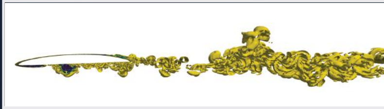
Simulation prediction of turbulent, cavitating flow over the hydrofoil based on the LCC experiment conditions
