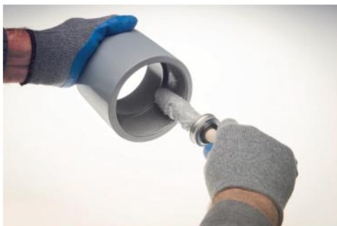
Apply cement to ID of pipe
