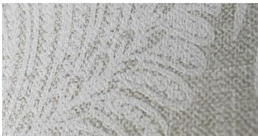
Print Style: Rotary Screen/Hybrid Emboss Ink: White Matt Ink Raised Relief Substrate: Textured Non-Woven Paper
