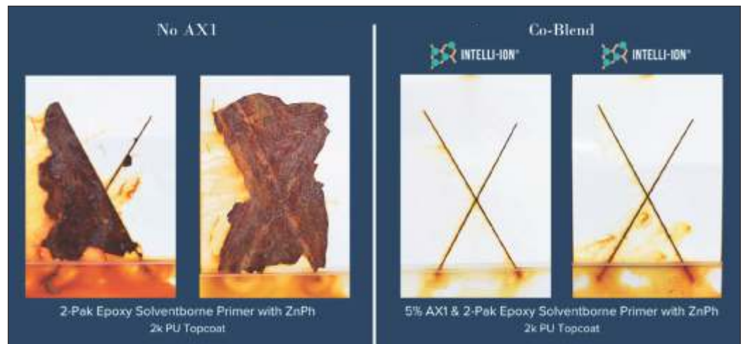
Figure 8: Solventborne 2-pak epoxy - 6000 hours of live coastal testing.
