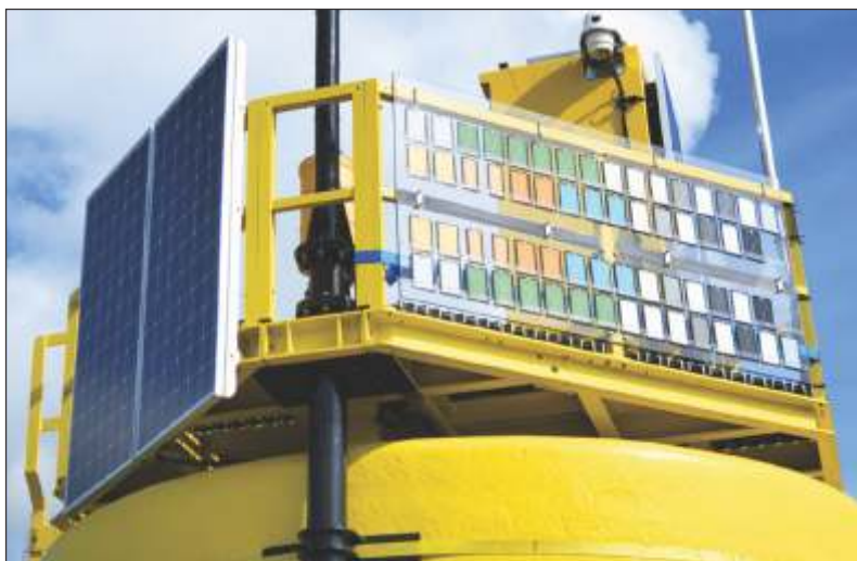
Figure 3: The final installation of the test rack onto the buoy.
