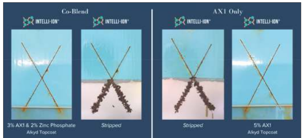
Figure 7: Solventborne alkyd - 6000 hours of live coastal testing.
