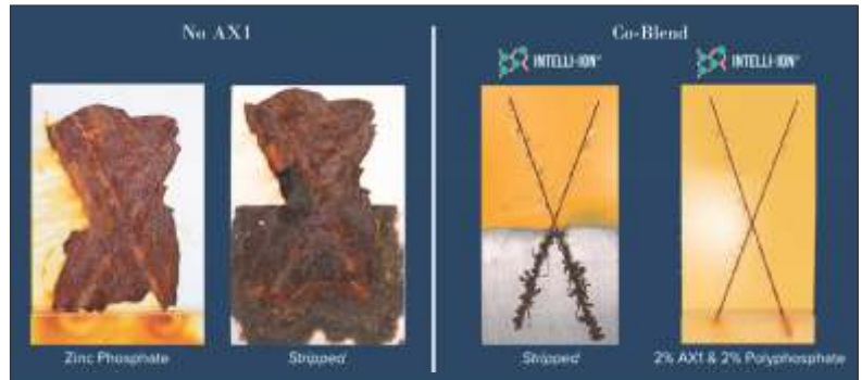
Figure 10: Solventborne 2-pak epoxy vs waterborne acrylic – 6000 hours of live coastal testing.
