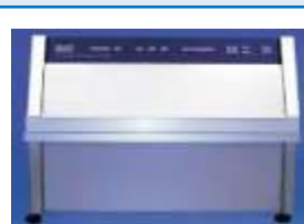
ACCELERATED WEATHEROMETER (QUV) ASTM G 154, ISO 16474
