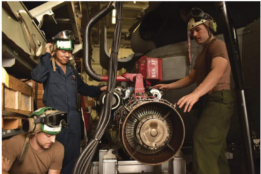
HSM-37 Detachment Four "Savages" to include AD2 Jacob Moore, AD1 Jeffrey Luk, and AEC Dominick Strona prepare to replace the #1 engine for Easyrider 36 in USS Michael Murphy's port hangar.
