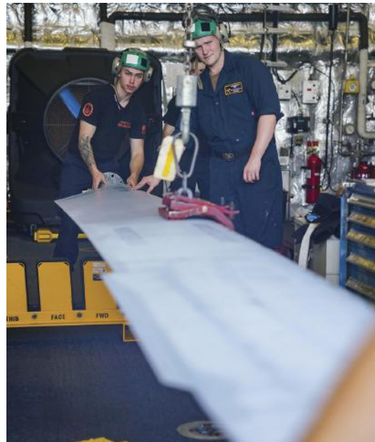
Aviation Machinist's Mate 1st Class Alexander Rauchfuss, right, and Aviation Electronics Technician 2nd Class Jordan Van Valkenburg, both assigned to HSM-35, guide a helicopter blade into a rack for maintenance in the hangar bay aboard USS Oakland (LCS 24). U.S. Navy photo by Petty Officer 2nd Class Sang Kim, USN.
