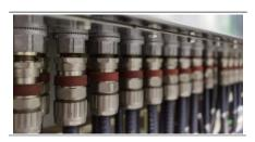
As cable diameter is approx. half of standard cables, all accessories like cable glands, high expensive offshore connectors and cable trays can be chosen smaller and therefore reduce cost and additional weight and space.
