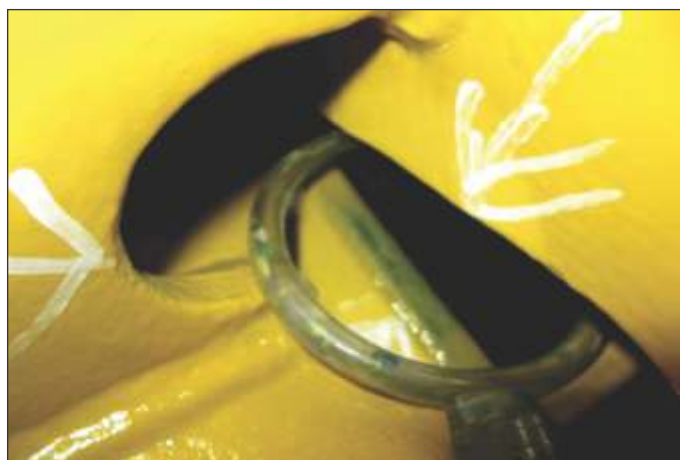
This image shows the effectiveness of BOA's self-indication; areas of low thickness can be found visually even in areas where thickness gauges cannot be used.
