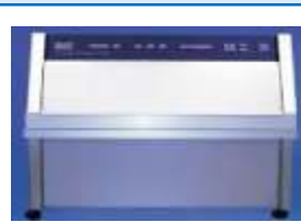
ACCELERATED WEATHEROMETER (QUV) ASTM G 154, ISO 16474
