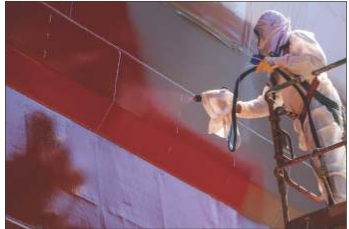
Electrostatic application of paint provides higher transfer efficiency than airless spraying, resulting in sustainability benefits.
