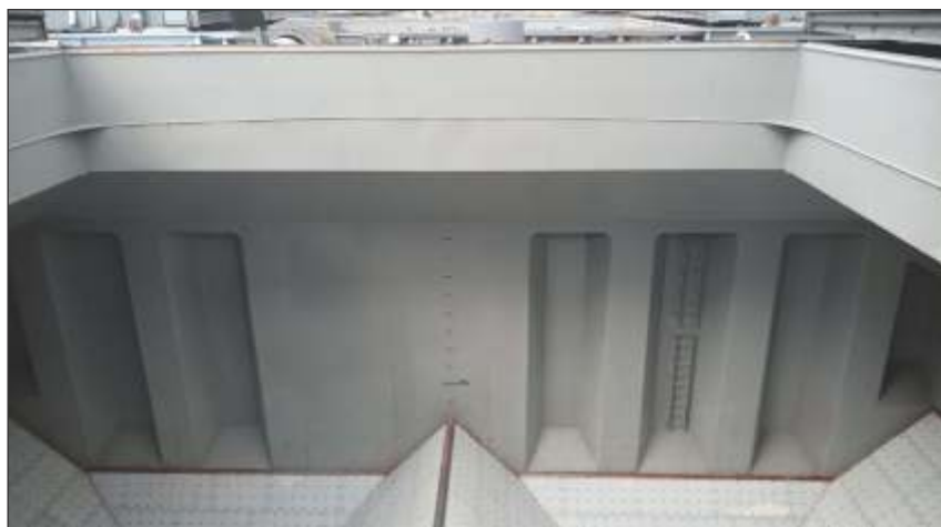
NEOGUARD coating system from Nippon Paint Marine was considered the only viable option, because the bulker Starnes carries crushed stones and other aggregates; the holds required a very tough coating to withstand mechanical impact, abrasion and prevent corrosion.
