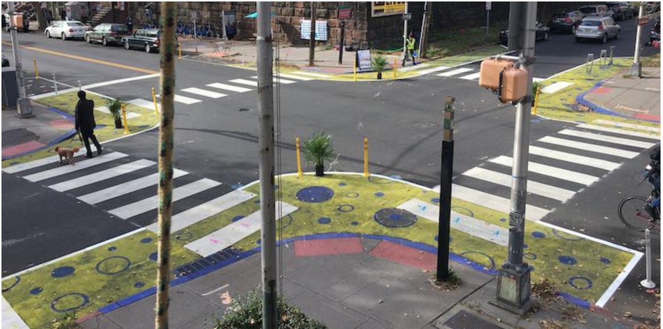
Figure 38: Shrinking intersections to improve pedestrian safety
