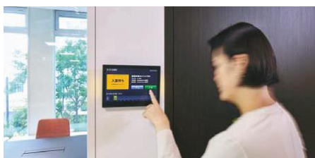
Room Display Terminal 01 terminal is installed at each meeting room to manage check-in and check-out. A speaker can also be installed in each room to play an alert
