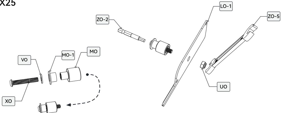
Install the louvre cover on two ends of the installed louvres and the spindle louvre.
