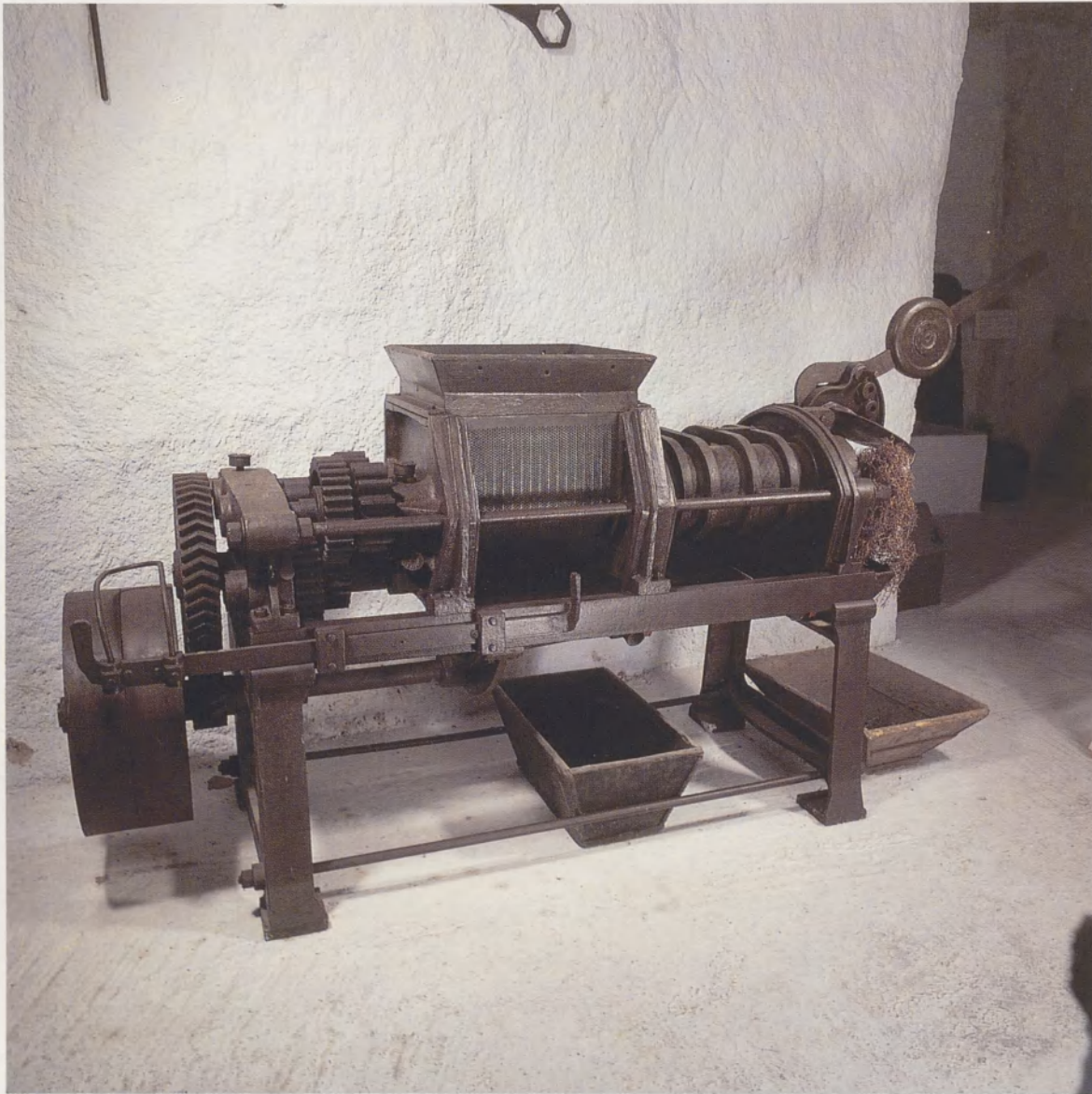
Fig. 37 Continuous metal screw winepress, among the first to be brought to the island (Santorini Wine Museum).
