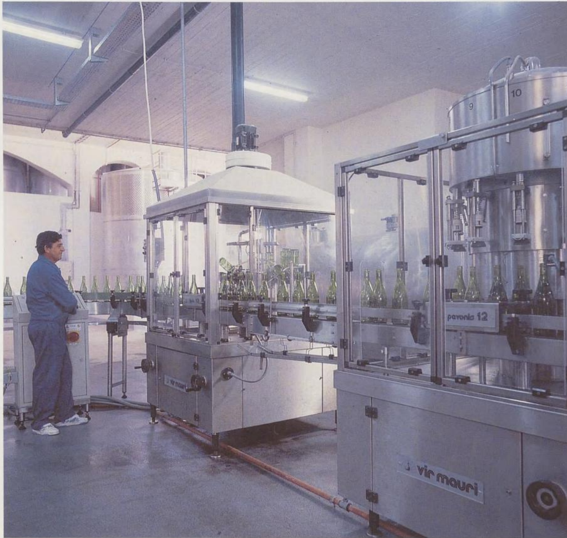
Fig. 81 The automated wine-bottling plant at the winery of the 'Union' of co-operatives.
