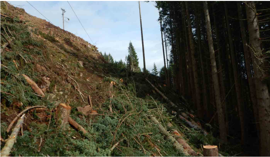
- Felled trees and logs awaiting to be choked and extracted by the cable crane
