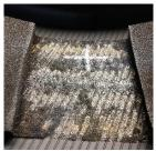
Complete the internal inspection and repair the tire per USTMA recommendations and procedures. Use a patch and plug, which seals the inner liner to prevent loss of inflation and keeps moisture out. It is not necessary to replace foam material that was removed and may be recycled with other scrap tires.
