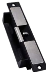
Stainless steel, mortise, fail-safe/secure, monitored, 12/24V AC/DC
