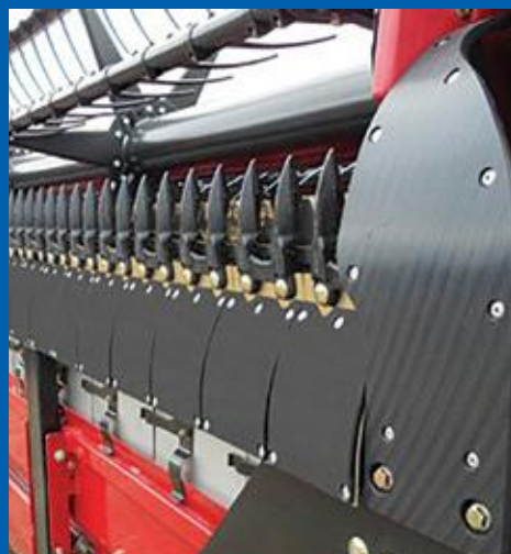
Predrilled & Counterbored Holes Protect Hardware. All Hardware is Included with Skid Shoes.
