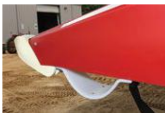
Inside & Outside Snouts with cutout for Height Control Sensor for Case IH 2200/2400/3200/3400
