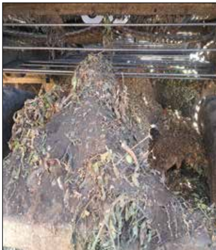
Dirt, mud and plant debris found on a tomato harvester. (UC Davis)
