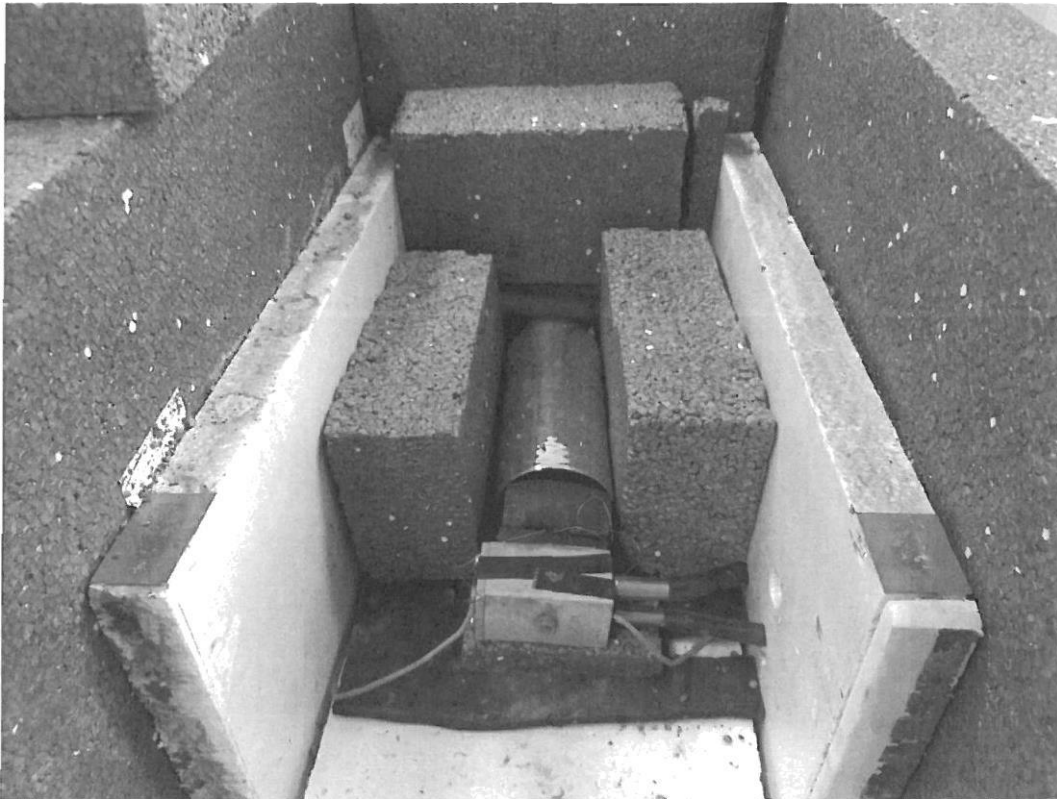
Figure 7. A heater-bracket-cooler unit in a Dewar flask and a thermally insulating body.
