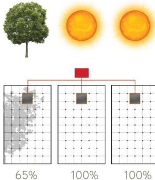
Shading Cuts Power by 35% On ONLY One Panel.
