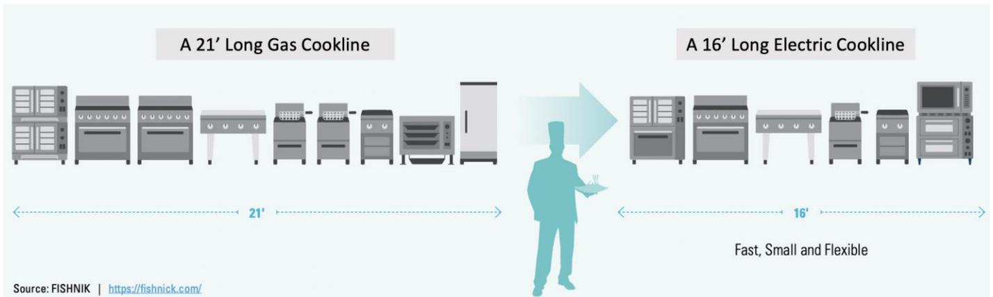
*Electric equipment takes less space to do the same amount of cooking. The easiest way for a restaurant to expand the kitchen's cooking capacity is to replace the gas equipment with electric and free up 30% more space.*
