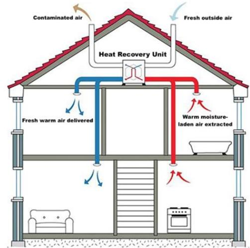
Figure 32: Heat Recovery ventilation system example.<sup>115</sup>
