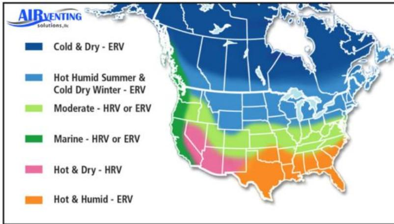
Figure 31: Choosing an HRV or ERV system based on location map.<sup>114</sup>
