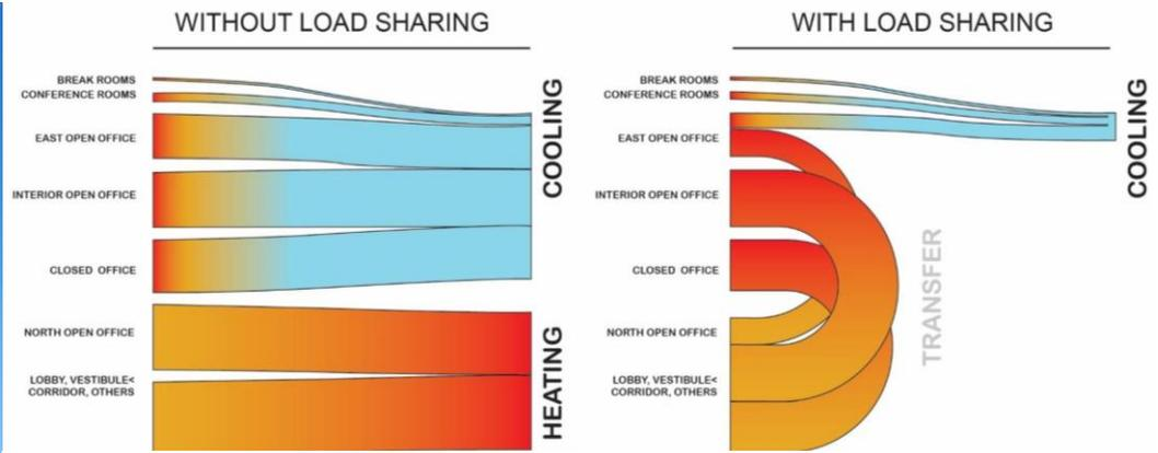
*Case Study: Multizone heat pumps can move heat from where it is being wasted to where it is needed. At 100 Avenue of the Americas in Manhattan, NY, they discovered that all of the winter space heating needed for exterior offices could be met with waste heat from air conditioning the interior core of the building during the winter. (Empire Building Playbook, April 2022. NYSERDA)*
