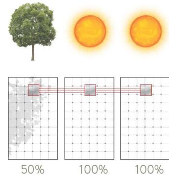
Shading Cuts Power by 50% On ONLY One Panel.
