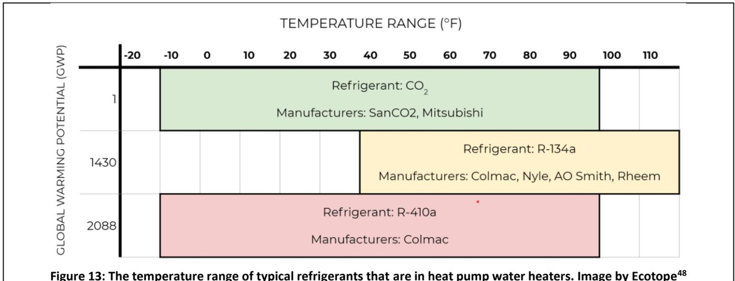
Figure 13: The temperature range of typical refrigerants that are in heat pump water heaters. Image by Ecotope<sup>48</sup>
