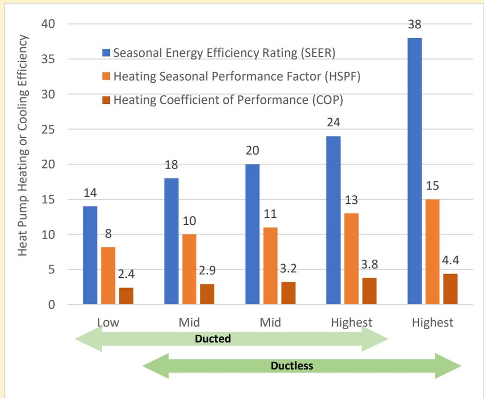
Figure 29: Typical heating and cooling efficiencies of heat pumps.
