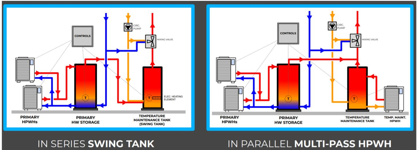
**Figure 14: The best practice designs of separating the temperature maintenance load from the primary hot water load. Image by Ecotope.<sup>49</sup>**
