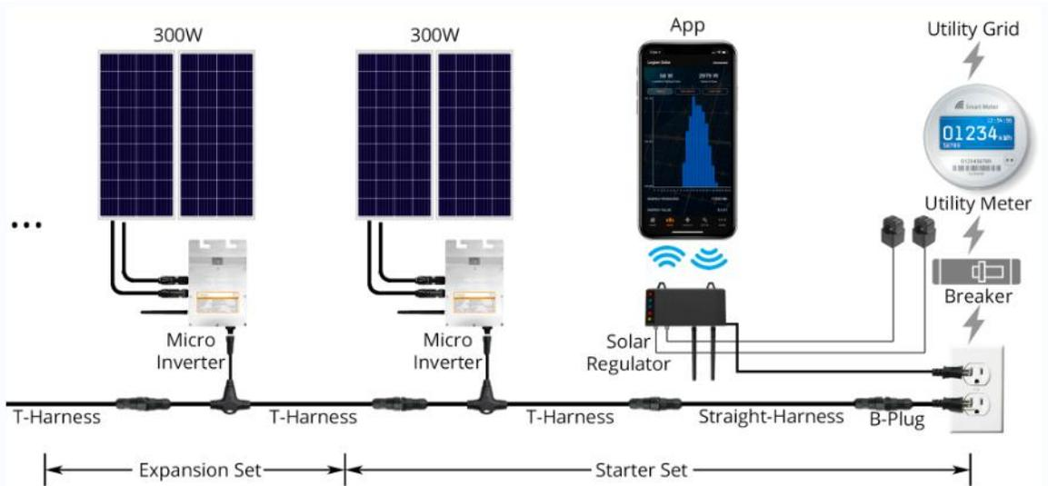
300W and can expand in stages of 300W depending on your budget and needs. Once your system is large enough to have excess energy to store during daylight, you can add expansion sets for nighttime consumption, this expansion set enables the solar panels to charge the batteries, solar panels to supply power to the micro inverters, and batteries to supply power to the micro inverters. No permit needed, plugs in the wall, solar alternative to a backup generator, and a bill saver.
