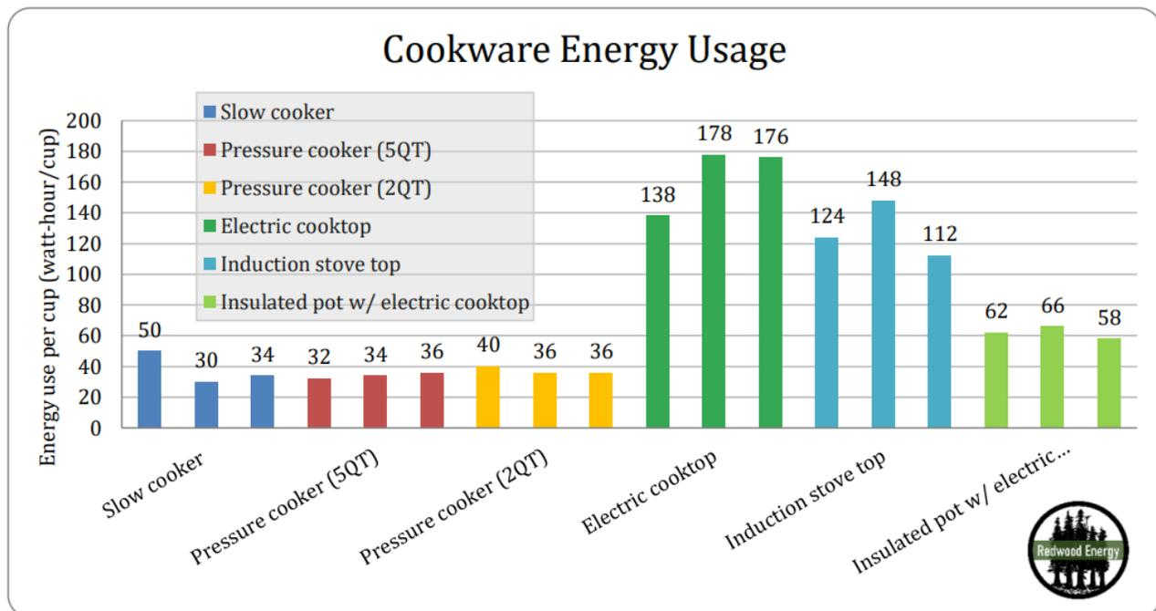
Figure 36: The results of the low power cooking study, the lowest energy use per cup were the pressure cooker and slow cookers.
