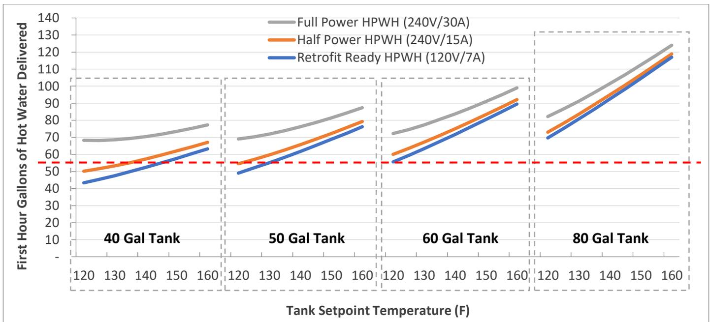
Approximate “first hour rating” (3gpm until the hot water runs out) based on the power of heat pump water heater, tank size and temperature setting.
