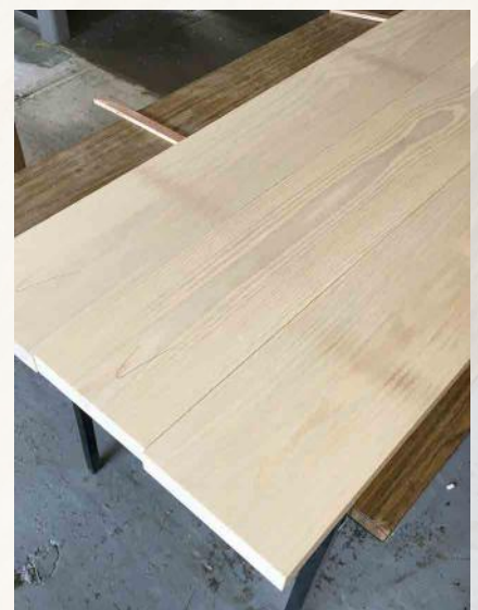
Clean ash boards - unacceptable sticker marks
