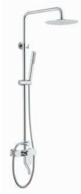
Conrad Shower Column with Shower Head Dia. 200 mm with Single Function Hand Shower & Hose with Foot Spout Height 1416 mm Min. Operating Pressure 1.5 bar MP
