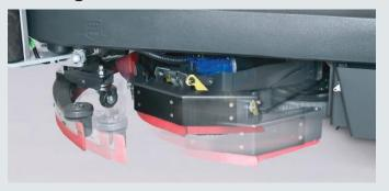
Retractable 4 inch (10 cm) offset disc deck enhances edge scrubbing and resists damage from accidental impact.
