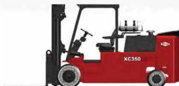
XC-350L Rated Capacity 35,000-lbs. (15,876 kg) 24-in. (610 mm) Load Center Alt. Capacity 31,000-lbs. (13,516 kg) 30-in. (762 mm) Load Center Alt. Capacity 28,000-lbs. (12,208 kg) 36-in. (914 mm) Load Center 98-in. (2,489 mm) Wheelbase
