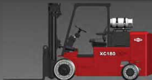
XC-180S & 180SL (SL models have lower overall height for container access) Rated Capacity 18,000-lbs. (8,165 kg) 24-in. (610 mm) Load Center Alt. Capacity 16,000-lbs. (7,258 kg) 30-in. (762 mm) Load Center Alt. Capacity 14,000-lbs. (6,350 kg) 36-in. (914 mm) Load Center 80-in. (2,032 mm) Wheelbase
