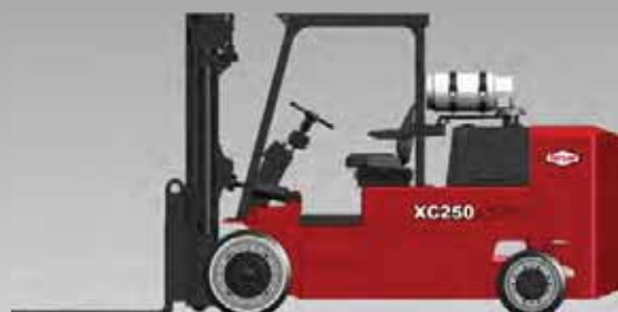
XC-250M Rated Capacity 25,000-lbs. (11,340 kg) 24-in. (610 mm) Load Center Alt. Capacity 22,000-lbs. (9,979 kg) 30-in. (762 mm) Load Center Alt. Capacity 20,000-lbs. (9,072 kg) 36-in. (914 mm) Load Center 88-in. (2,235 mm) Wheelbase
