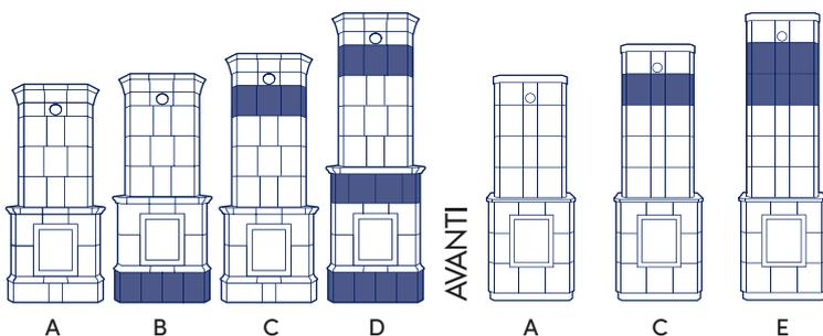
Height can be adjusted upwards or downwards in intervals of about 110 mm.
