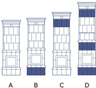
Height can be adjusted upwards or downwards in intervals of about 100 mm.
