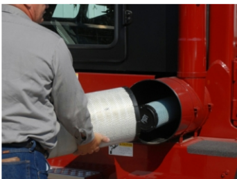
Donaldson Air Cleaner with Safety Element (Standard)
