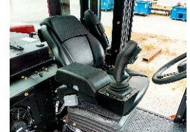
Fully Adjustable Air Ride Seat (Standard)
